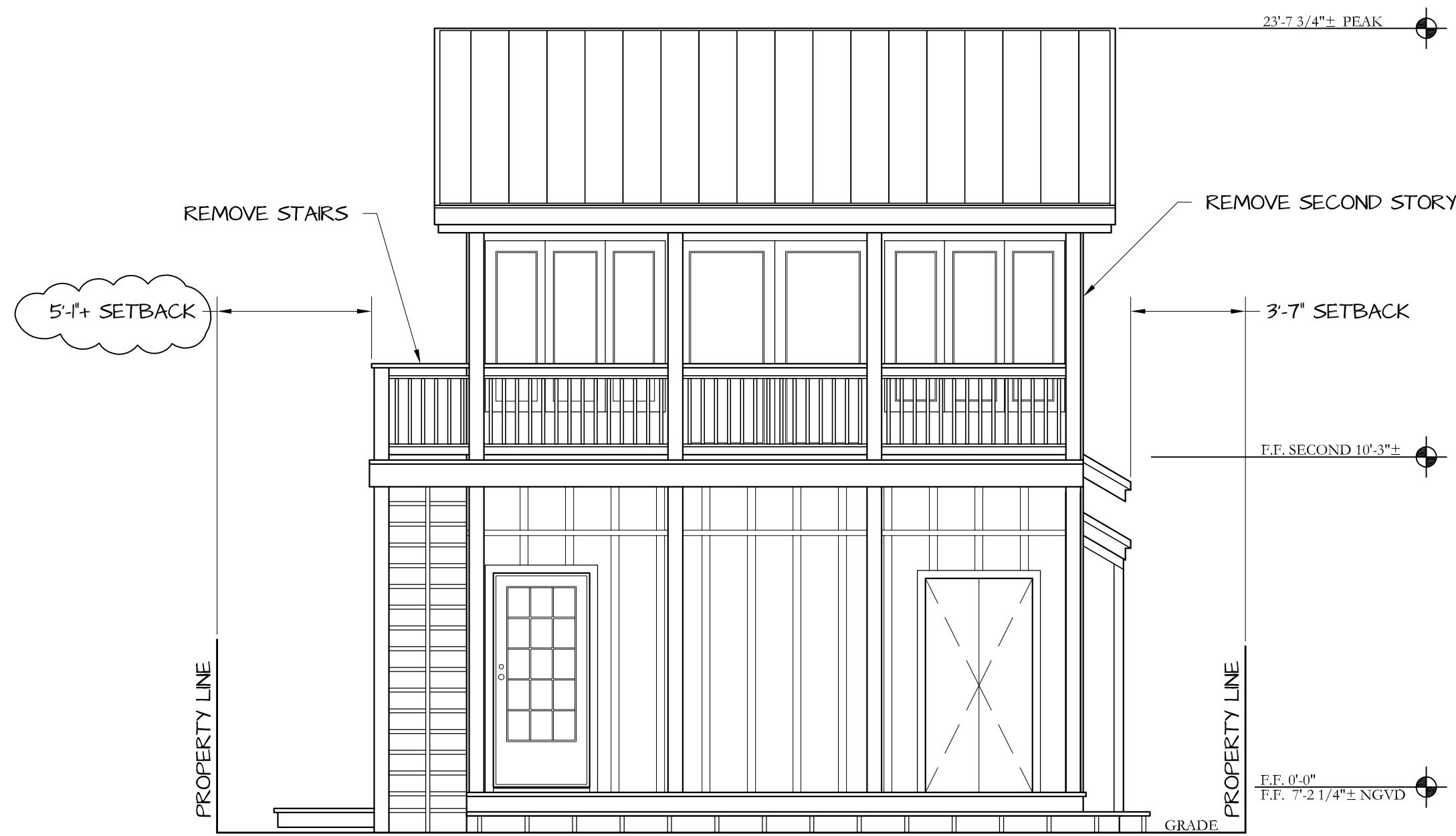
SOUTH ELEVATION (EXISTING) 1/4" = 1'-0"
