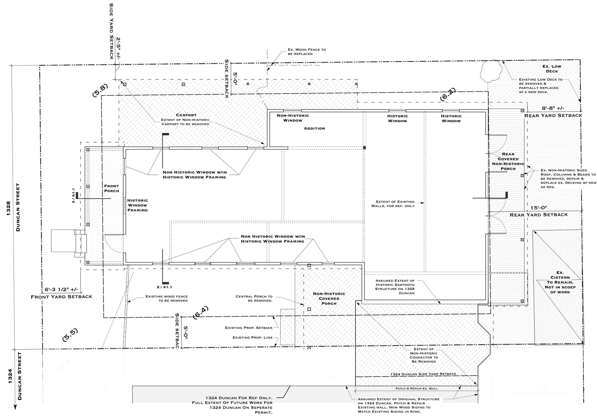
**1** EXISTING FLOOR / SITE PLAN + DEMOLITION
