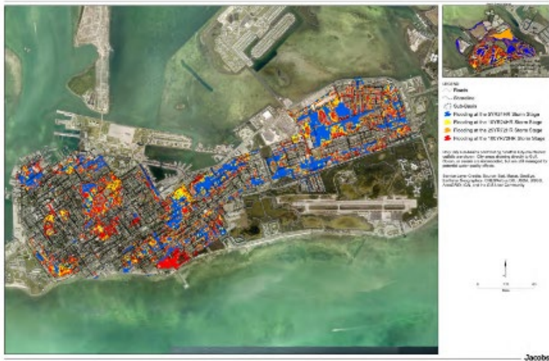
Figure 3-4. Predicted Stormwater Peak Elevations for Design Storms in Key West City of Key West 2013 Stormwater Master Plan
