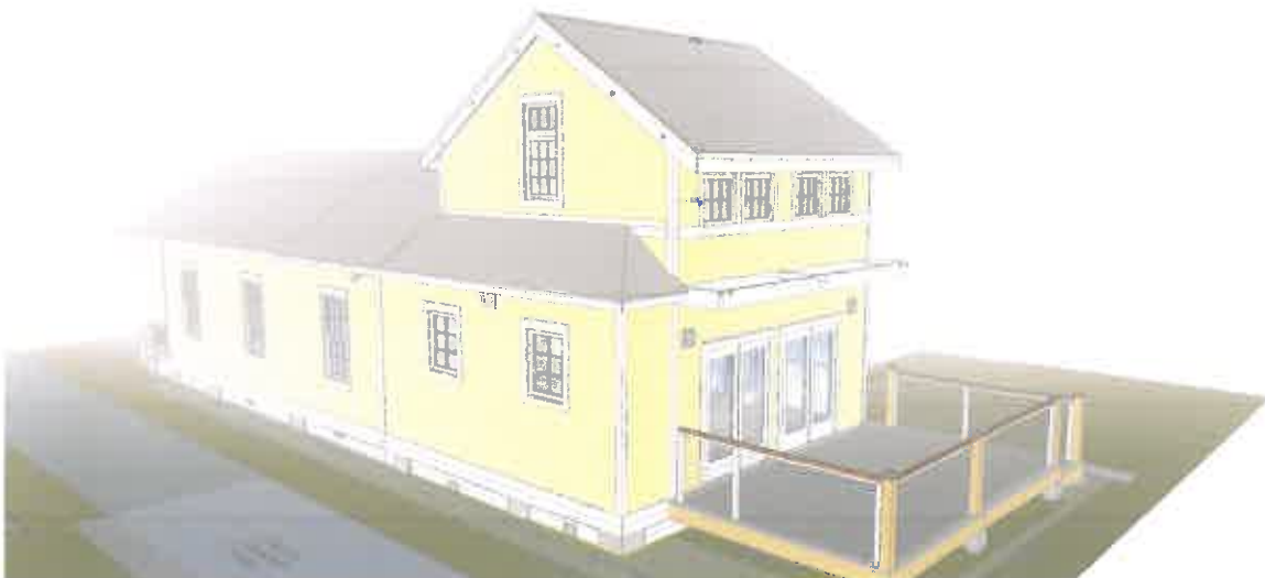
Drawing shows approved addition wall moved inside 5' Zoning Setback Line
