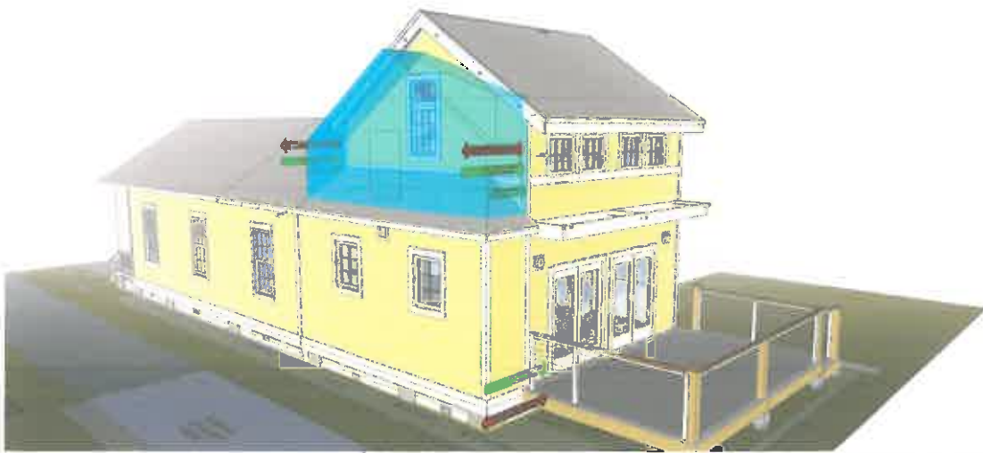
Drawing shows Approved 2 nd Floor Volume reduced to facilitate Fire Dept. Access
