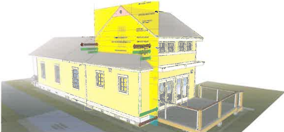
Drawing shows approved addition wall moved inside 5' Zoning Setback Line
