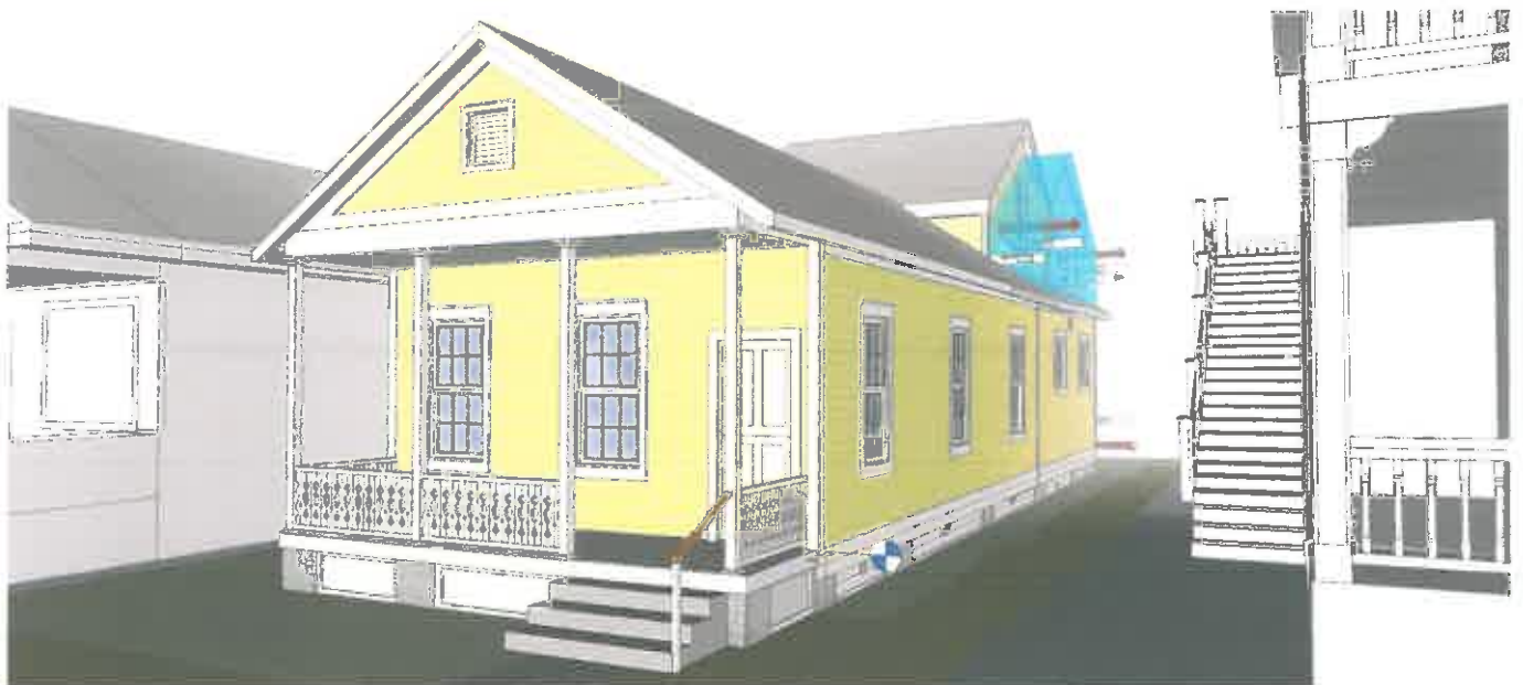
Removing encroaching 2 nd Floor Building Mass creates 5' clearance for Fire Access
