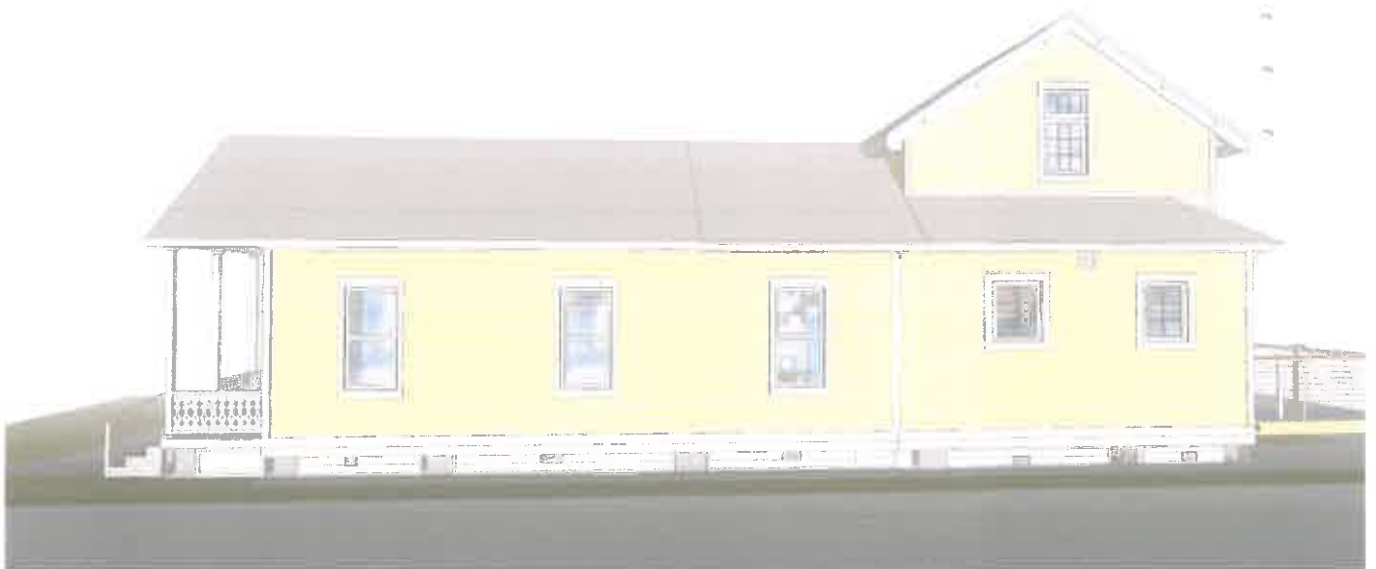
West Elevation shows changes to the roofline & new windows at the rear of building
