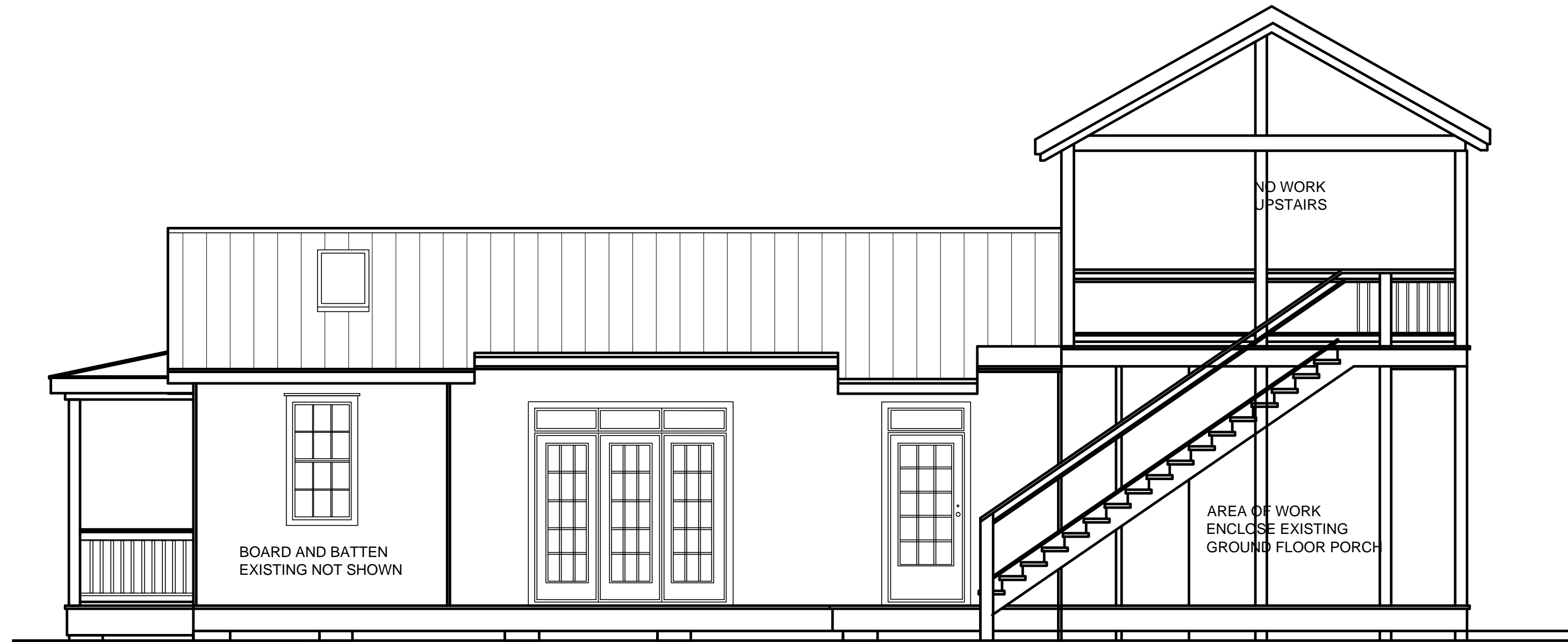
AS BUILT RIGHT ELEVATION 1" = 4'-0"
