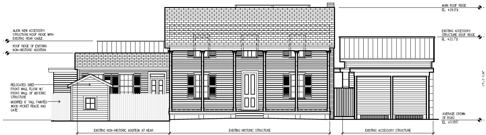
PROPOSED FRONT ELEVATION 3/16"=1'-0"
