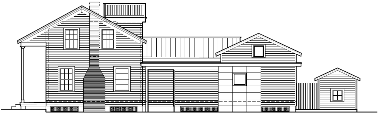
EXISTING STREET SIDE ELEVATION (VON PHISTER STREET) \frac{3}{16}"=1'-0"
