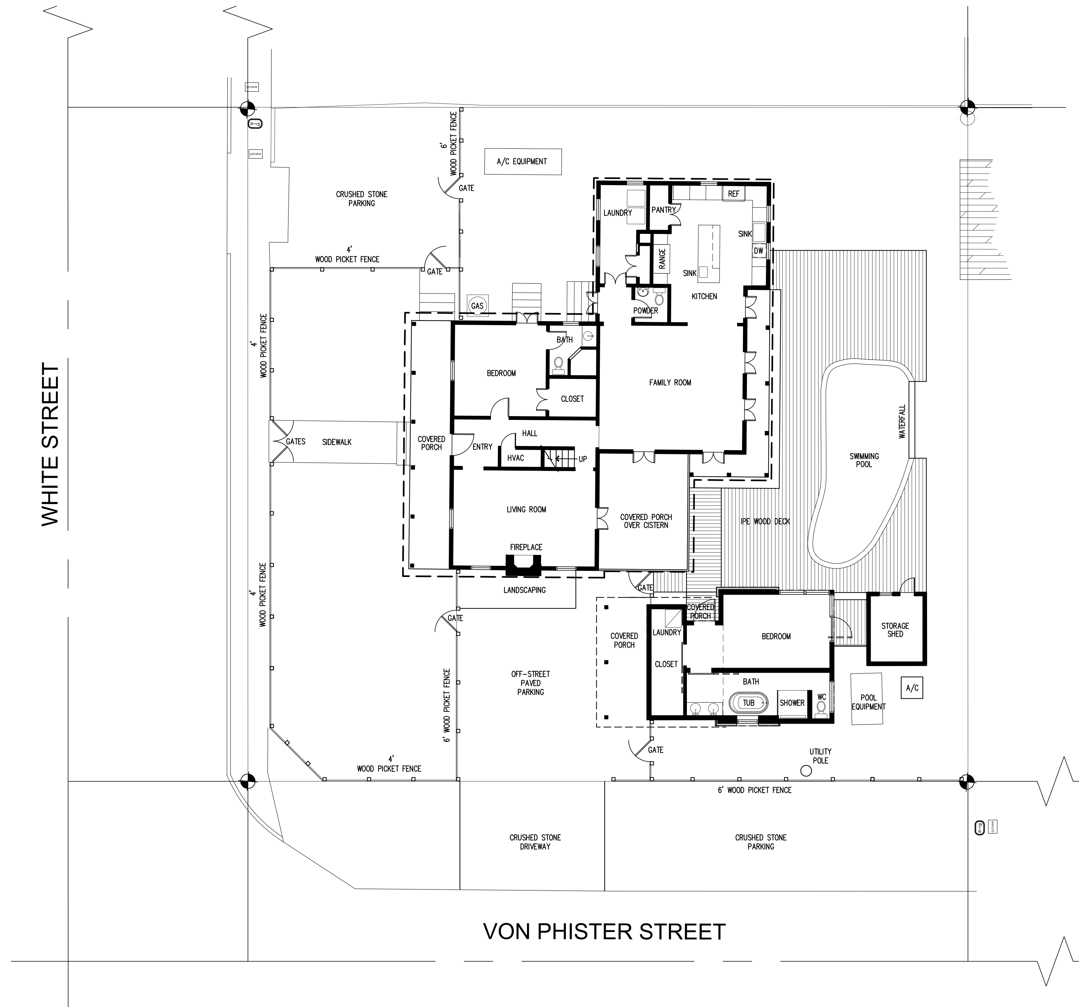
EXISTING SITE PLAN / FIRST FLOOR PLAN 1/8"=1'-0"
