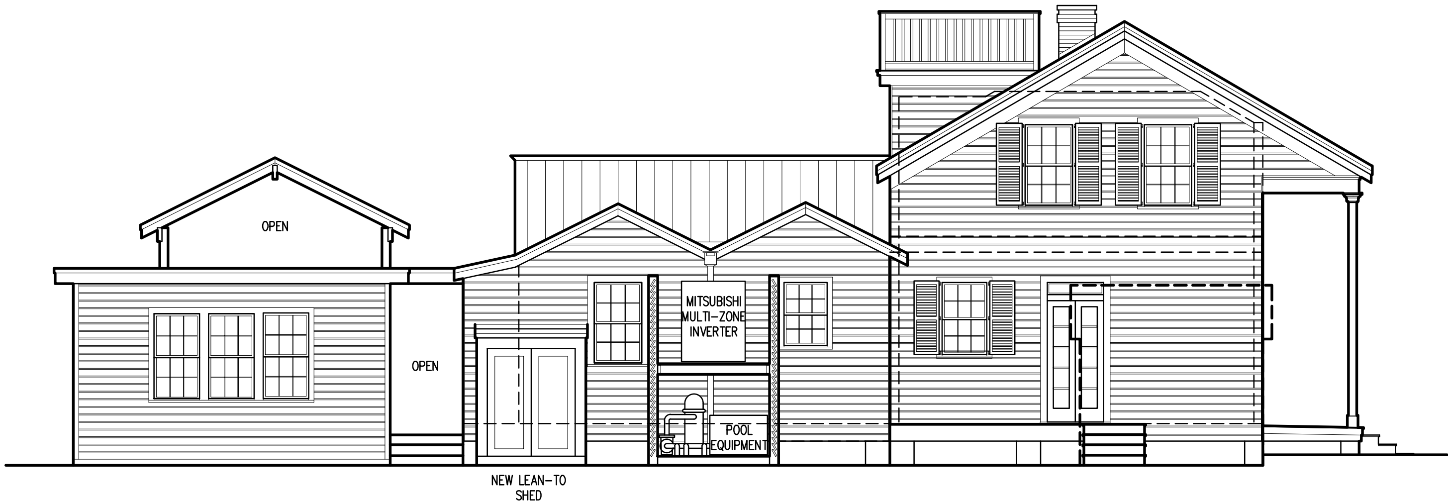
PROPOSED SIDE ELEVATION (FACING CHURCH) 3/16"=1'-0"
