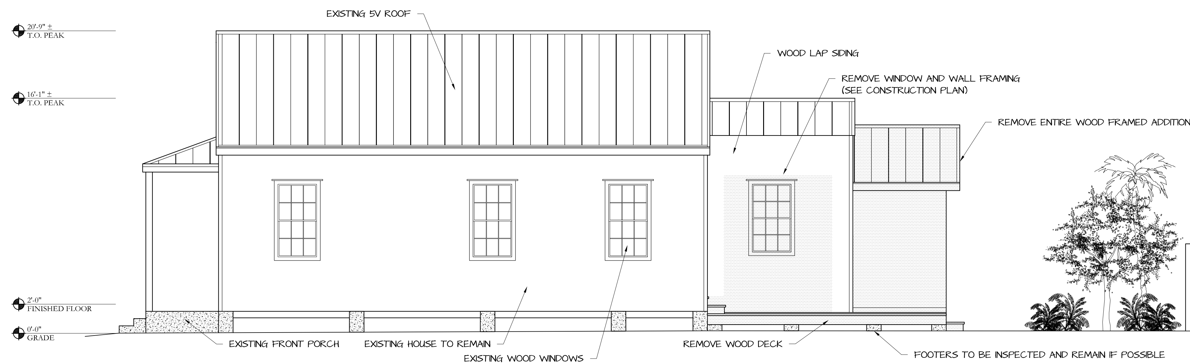
SOUTH ELEVATION (EXISTING) 1/4" = 1'-0"
