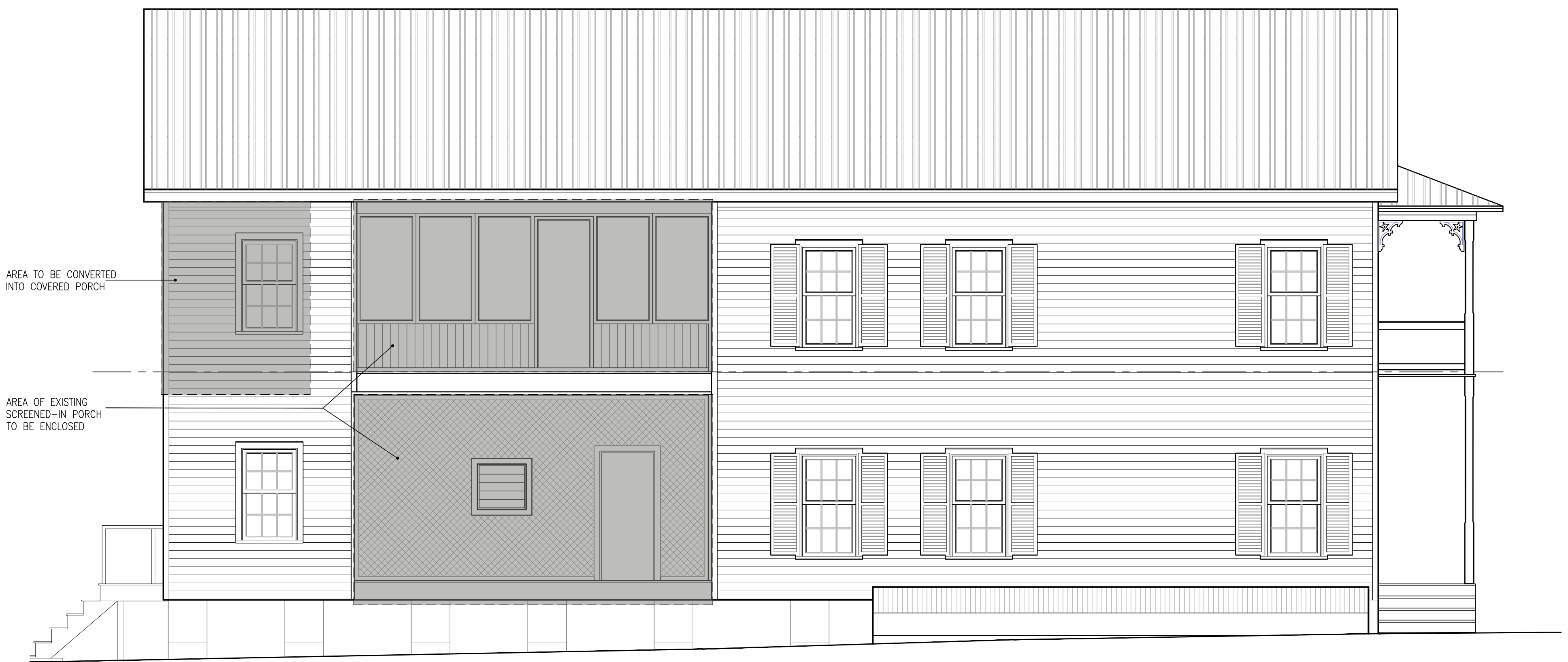
1 EXISTING NORTH ELEVATION / DEMO AE3.1 SCALE: 1/4"=1'-0"
