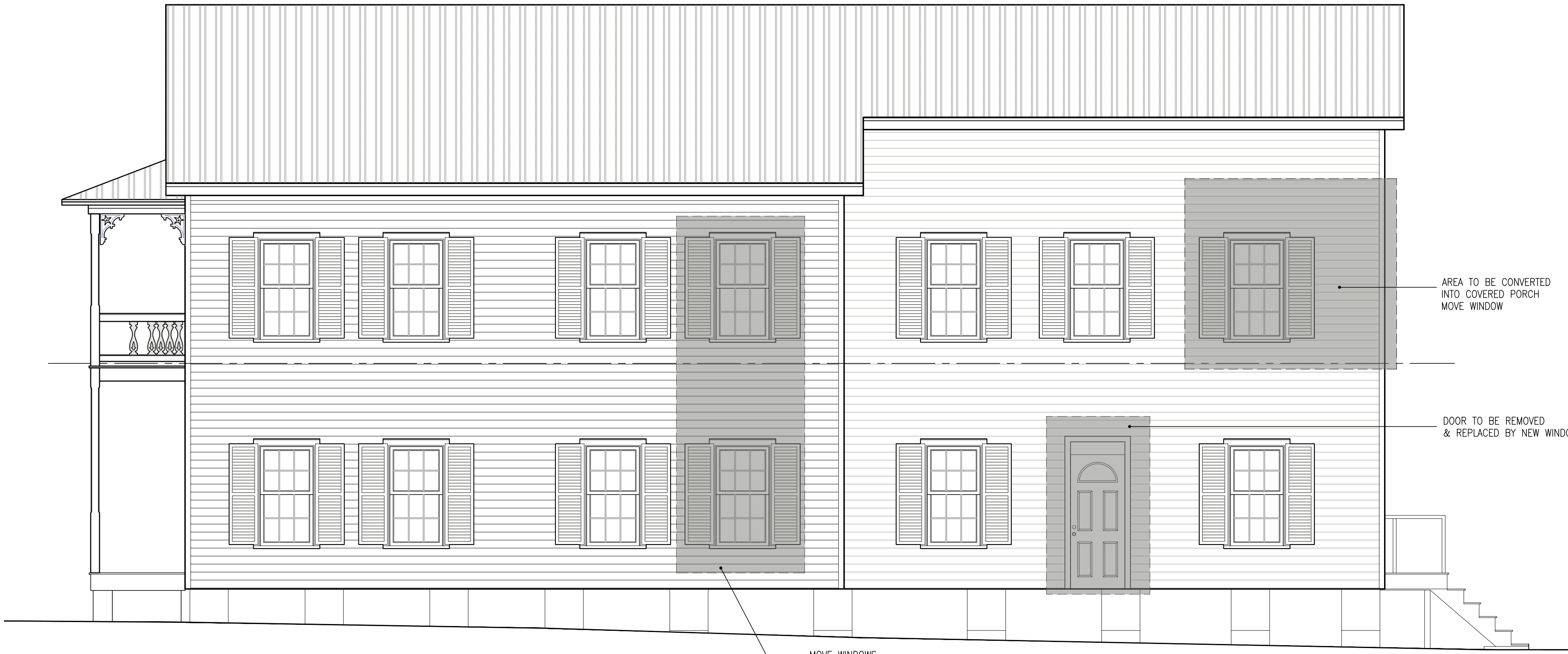
3 EXISTING SOUTH ELEVATION / DEMO AE3.1 SCALE: 1/4"=1'-0"
