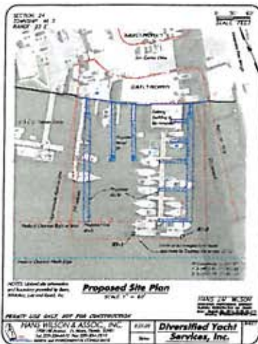
Proposed site plan drawing showing proposed docks overlain on aerial of existing docks.
