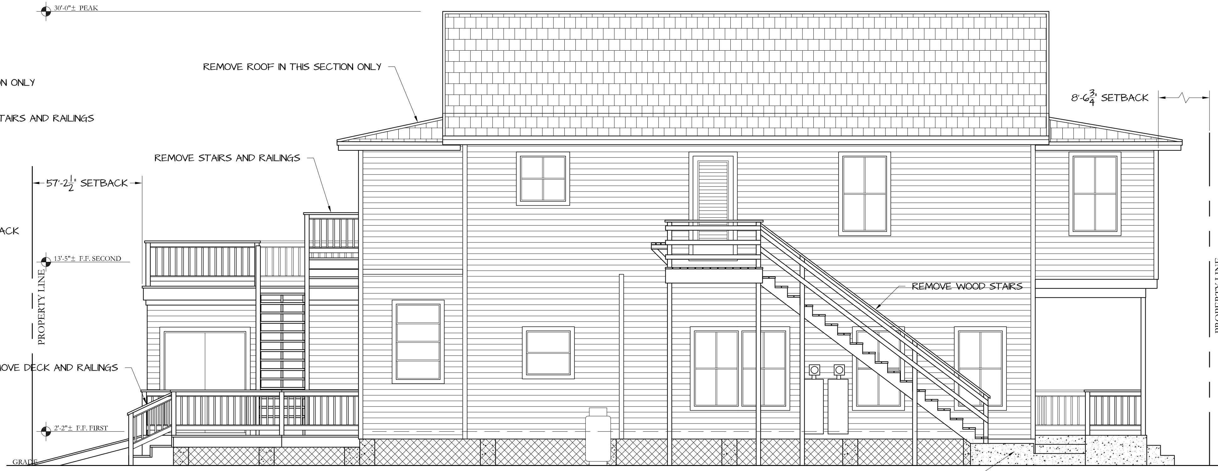
WEST ELEVATION (EXISTING) 1/4" = 1'-0"
