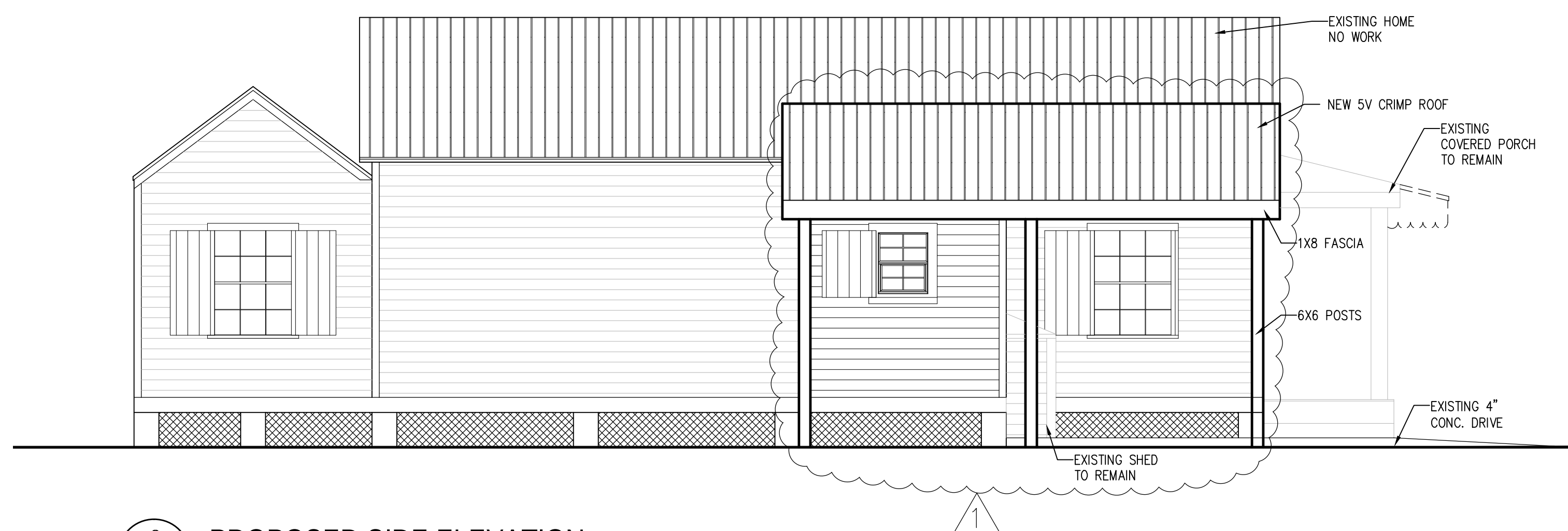
2 PROPOSED SIDE ELEVATION A-1 SCALE: 1/4"= 1'-0"
