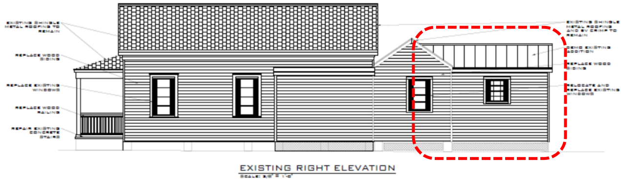
Existing Right Elevation, red dashed area to be demolished.
