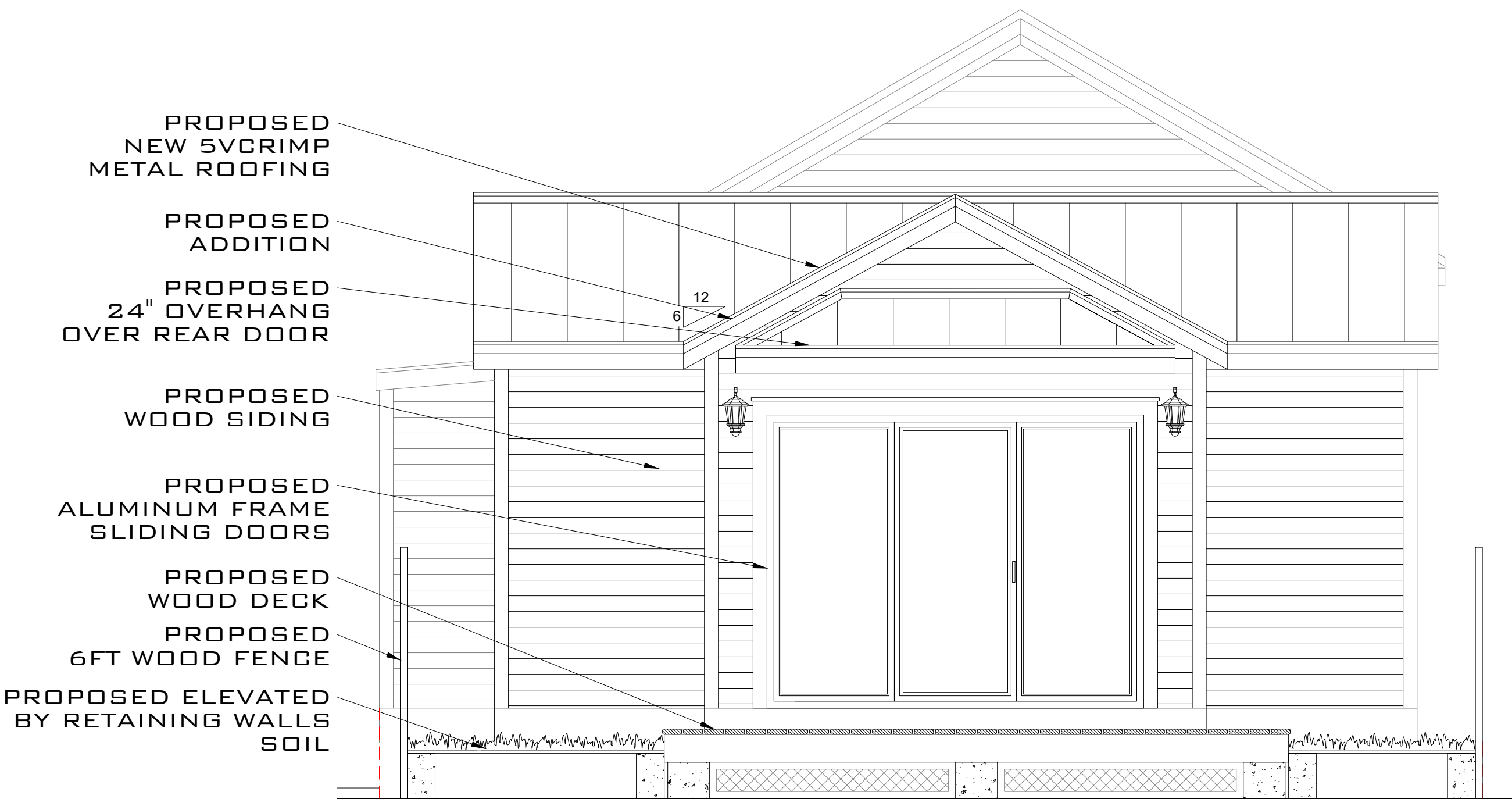
PROPOSED REAR ELEVATION SCALE: 3/8" = 1'-0"
