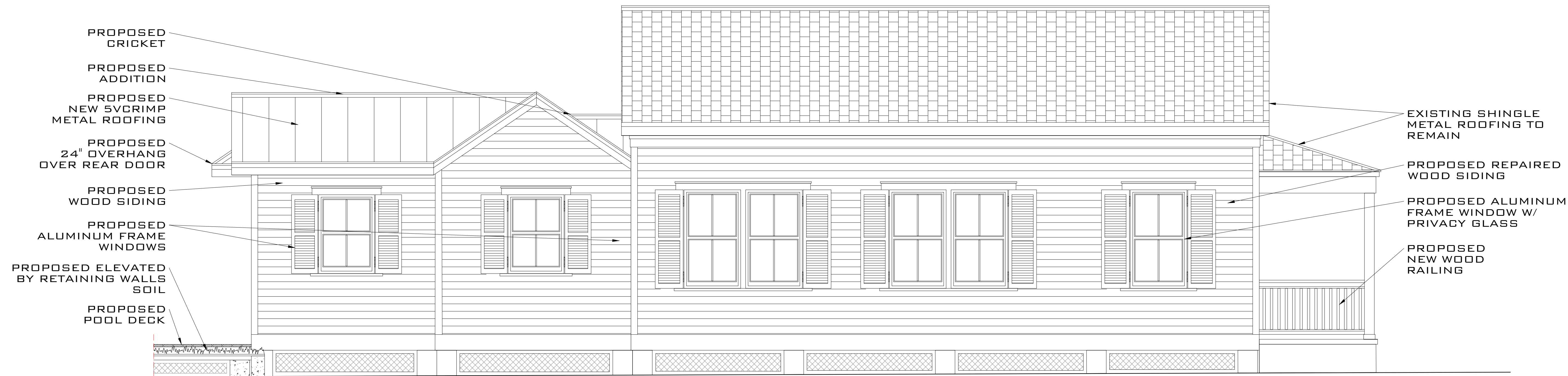
PROPOSED LEFT ELEVATION SCALE: 3/8" = 1'-0"
