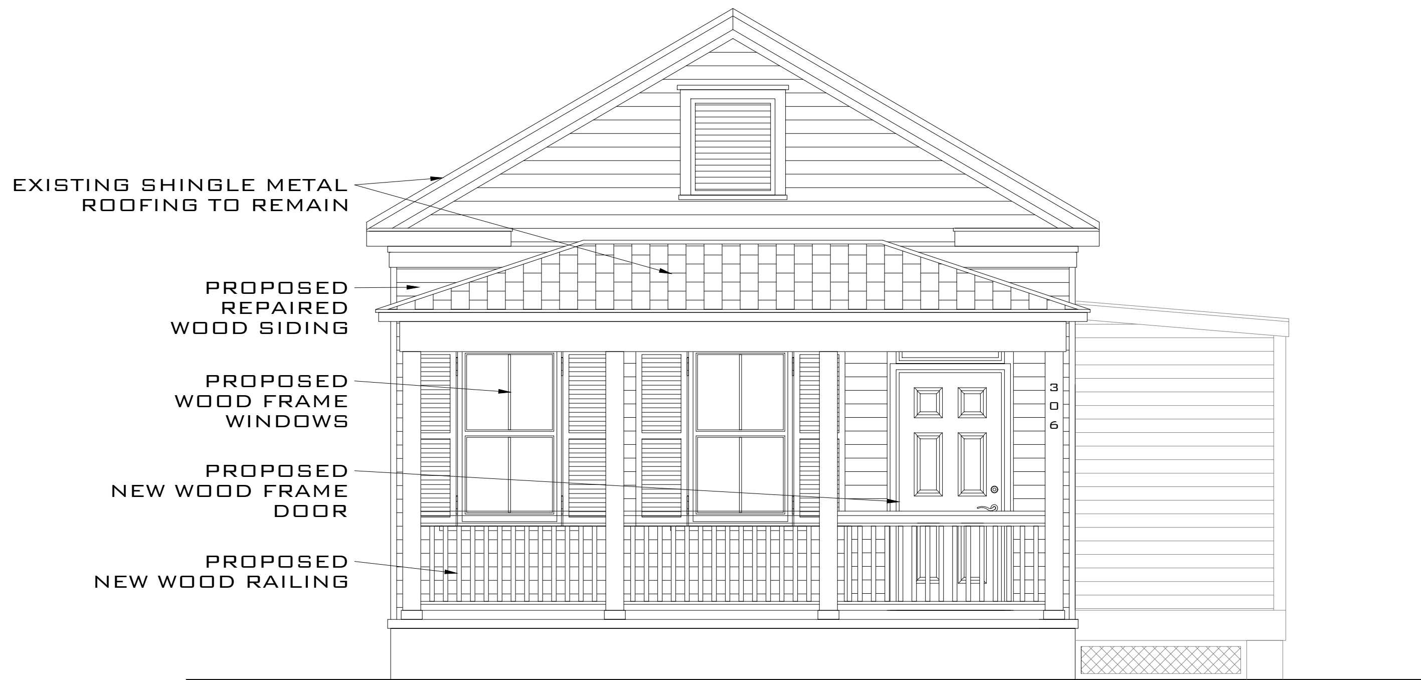
PROPOSED FRONT ELEVATION SCALE: 3/8" = 1'-0"
