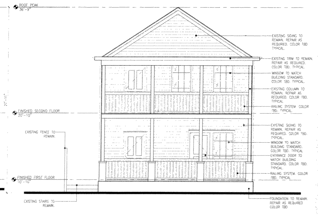
01 A3.6.1 BUILDING F - EAST ELEVATION (WHITEHEAD STREET) SCALE: 1/4"=1'-0"
