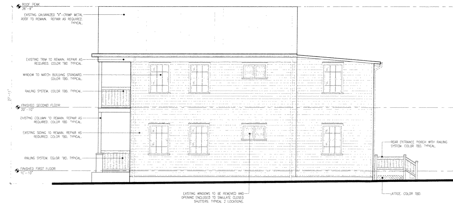
03 A3.6.1 BUILDING F - NORTH ELEVATION SCALE: 1/4"=1'-0"
