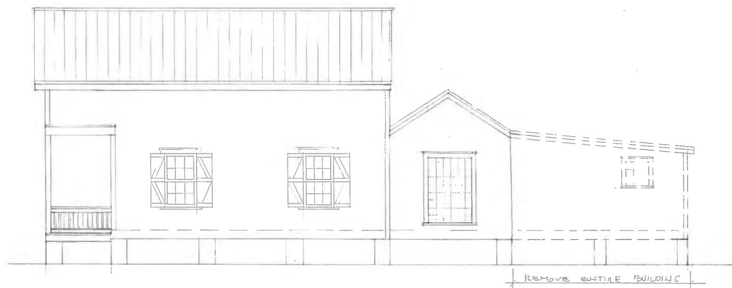
EXISTING/EAST ELEVATION (SIDE ELEVATION) DEMOLITION 1/4" = 1'-0"
