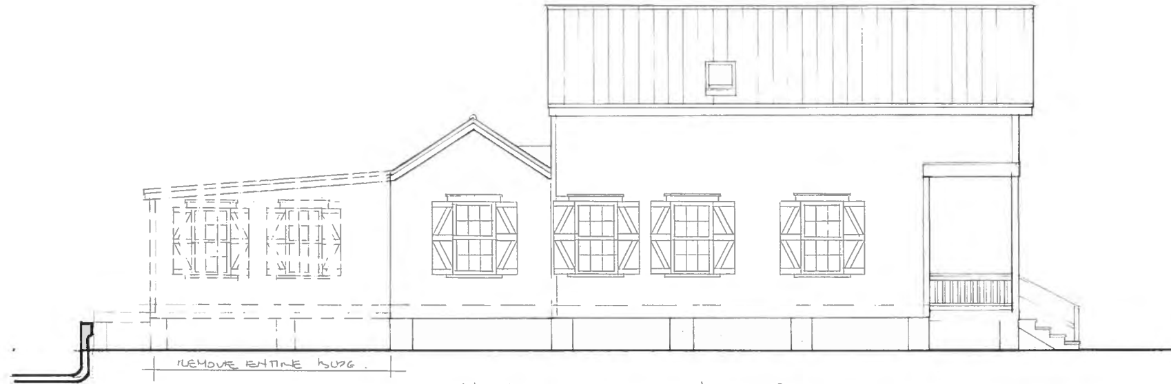
EXISTING/EAST ELEVATION (SIDE) DEMOLITION 1/4" = 1'-0"
