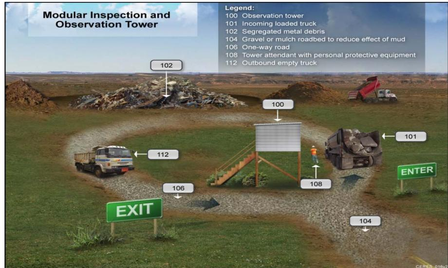
After inspection, the material will be forwarded to the tipping area supported by a wheel loader with rake and laborers. The laborers will inspect the debris and remove any contaminants. Contaminants that are hazardous will be handled by the Hazardous Toxic Waste Specialist, staged in the Hazmat containment area, and disposed of in accordance with federal, state, and local requirements. Other contaminants, such as metal, will be segregated accordingly.
