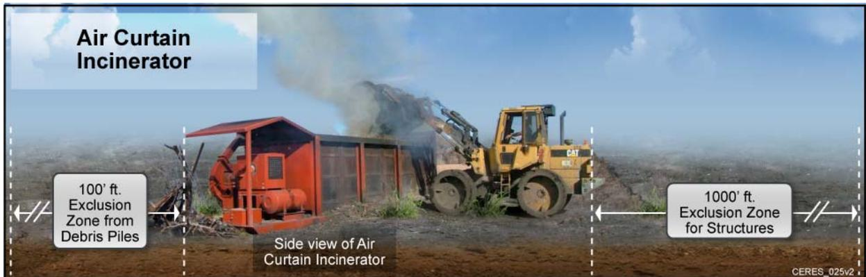
The Air Curtain will be operated at least 100 feet from any stockpile of debris and at least 1,000 feet from any occupied structure. Prior to removal of ash debris from the air curtain incinerator pit, the material will be wetted. Ash stockpiles will be at least 100 feet away from any debris stockpiles.
