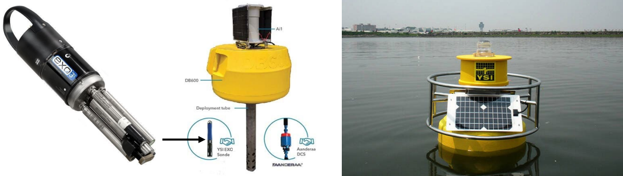
Figure 4. The DB-600 water quality monitoring buoy system with a current meter and YSI Exo data sonde with up to six water quality monitoring sensors.
