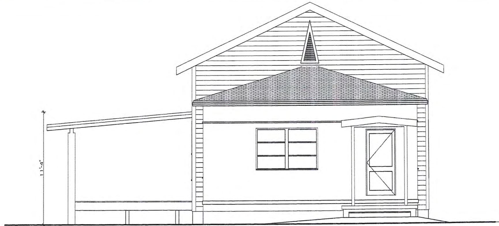
OPTION 001 EXISTING FRONT ELEVATION SCALE : 3/16"=1'
