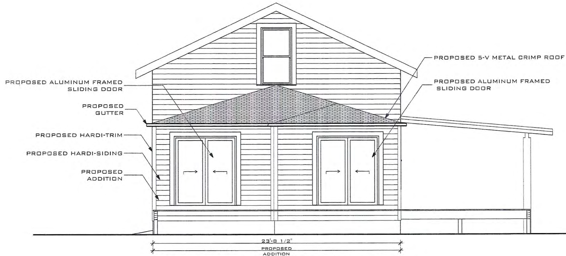
CASE STUDY 003 PROPOSED REAR ELEVATION SCALE : 3/16" = 1'
