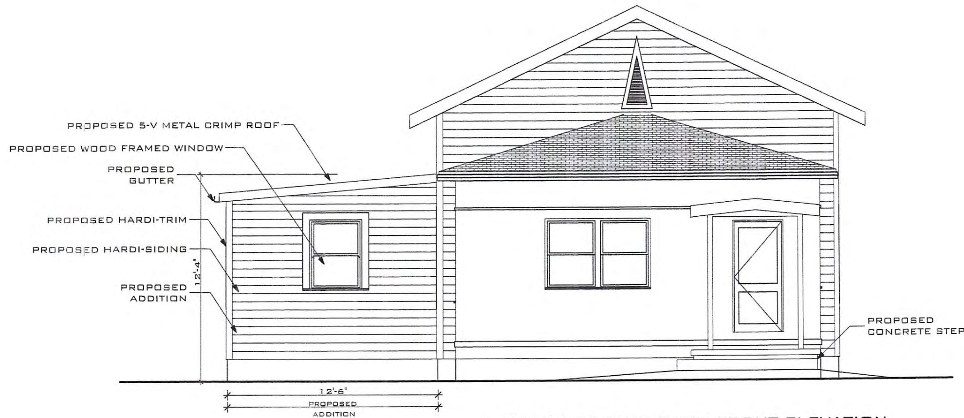
OPTION 002 PROPOSED FRONT ELEVATION SCALE : 3/16" = 1'
