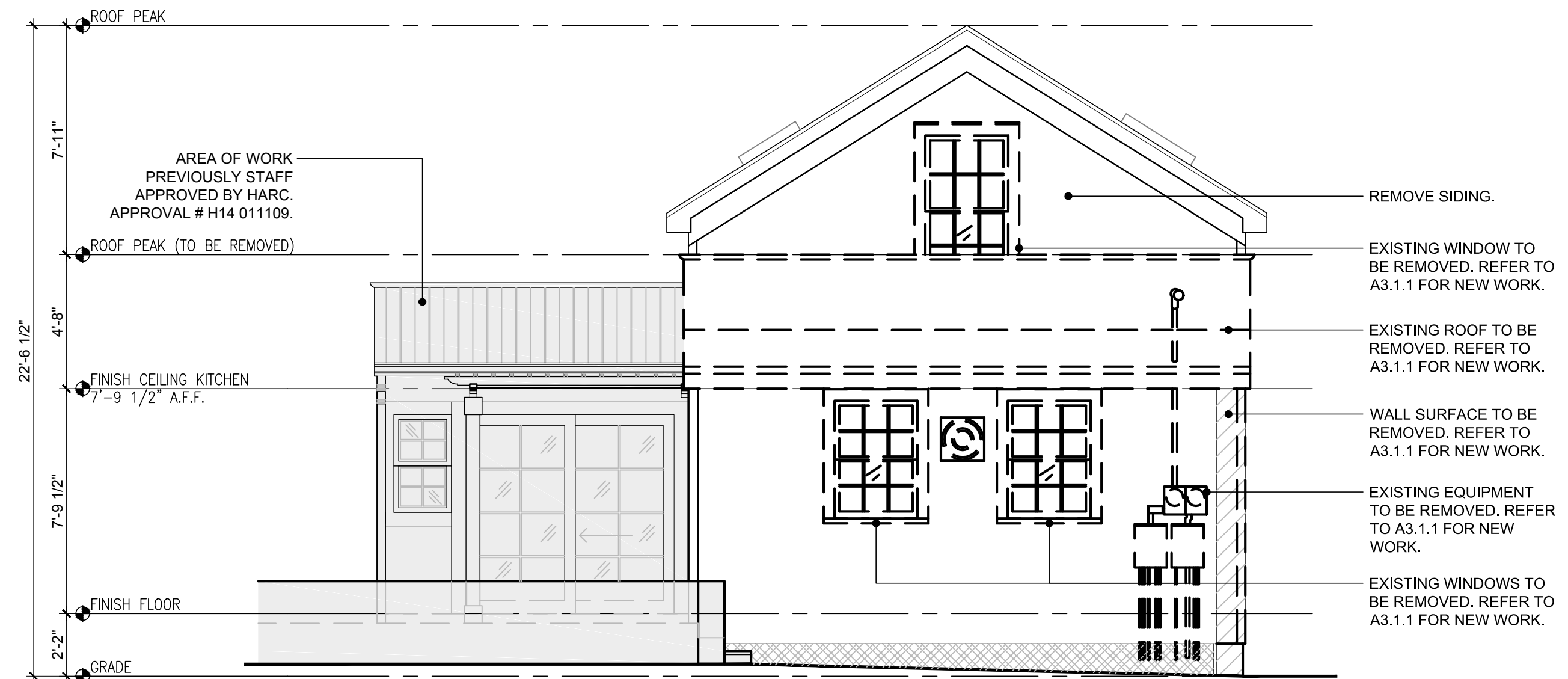
3 DEMOLITION SOUTH ELEVATION SCALE: 1/4"=1'-0" GRAPHIC SCALE: 1/4" = 1'-0"
