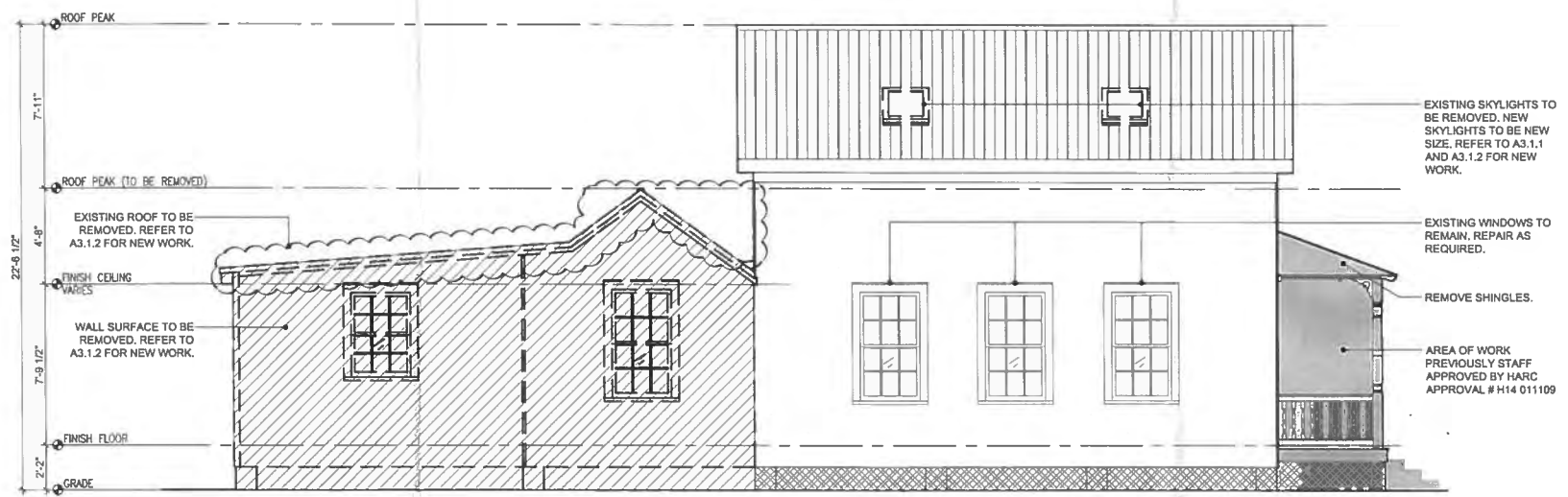
2 DEMOLITION EAST ELEVATION SCALE: 1/4"=1'-0"
