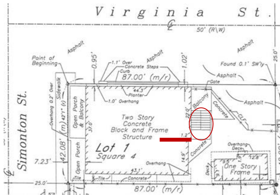
Proposed demolition for non-historic portions of the house is highlighted in red.
