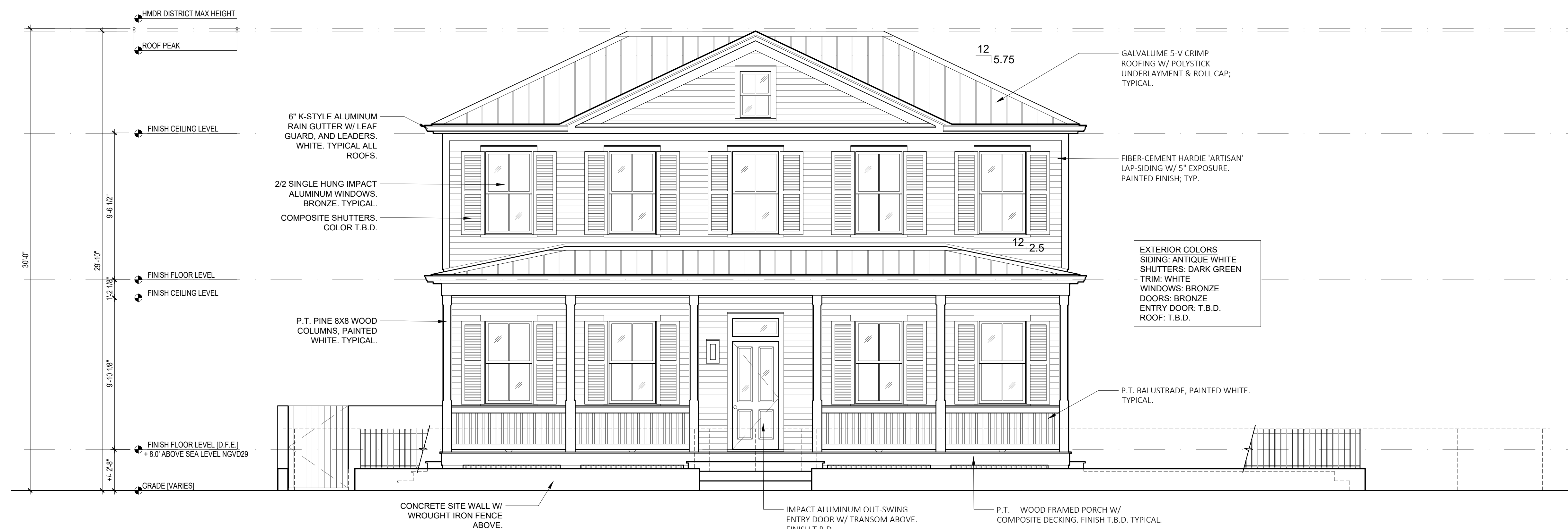
1 PROPOSED SOUTH ELEVATION [FRONT AT STREET] SCALE: 1/4" = 1'-0"
