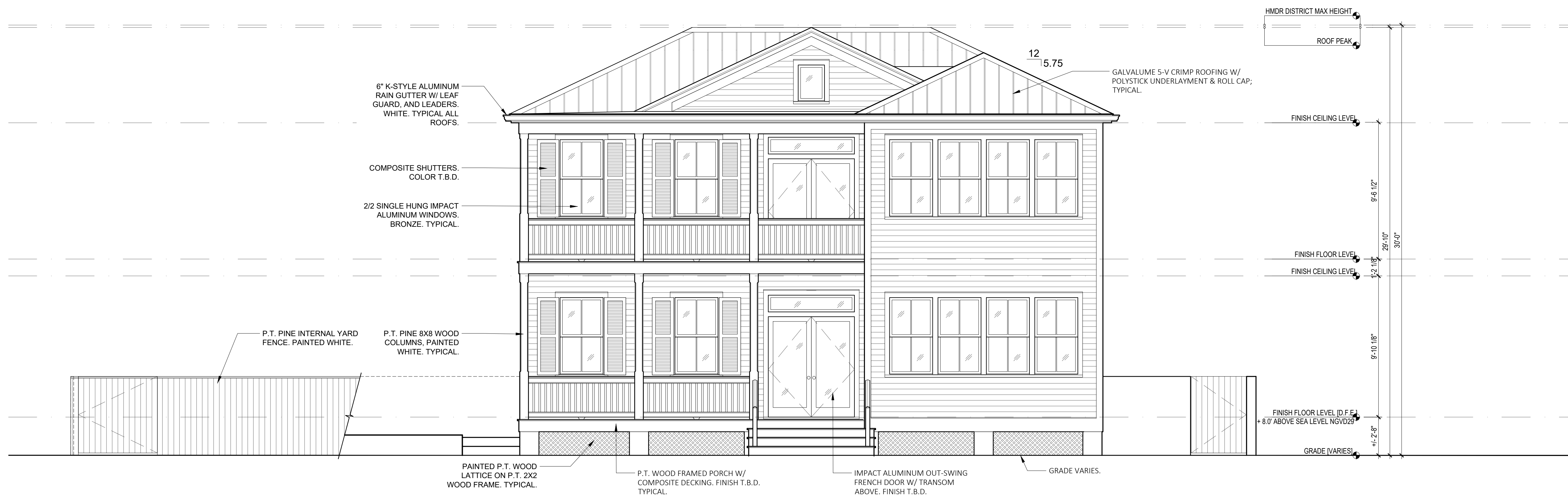
2 PROPOSED NORTH ELEVATION [REAR] SCALE: 1/4" = 1'-0"
