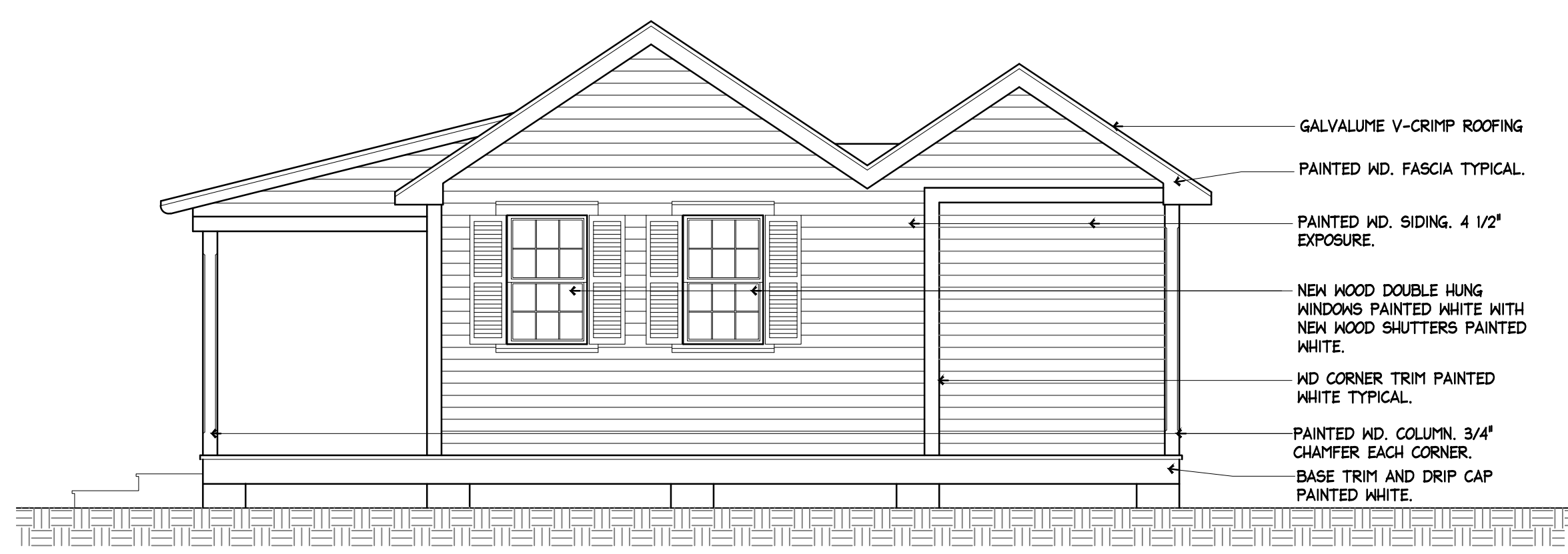
1 BUILDING #3 (STUDIO) NORTH ELEVATION SCALE: 1/4"=1'-0"
