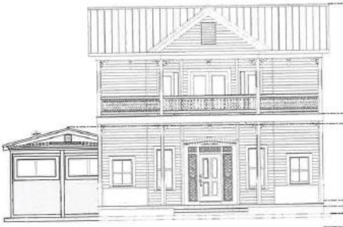
Existing Front Elevation with main structure (shed already demolished).
