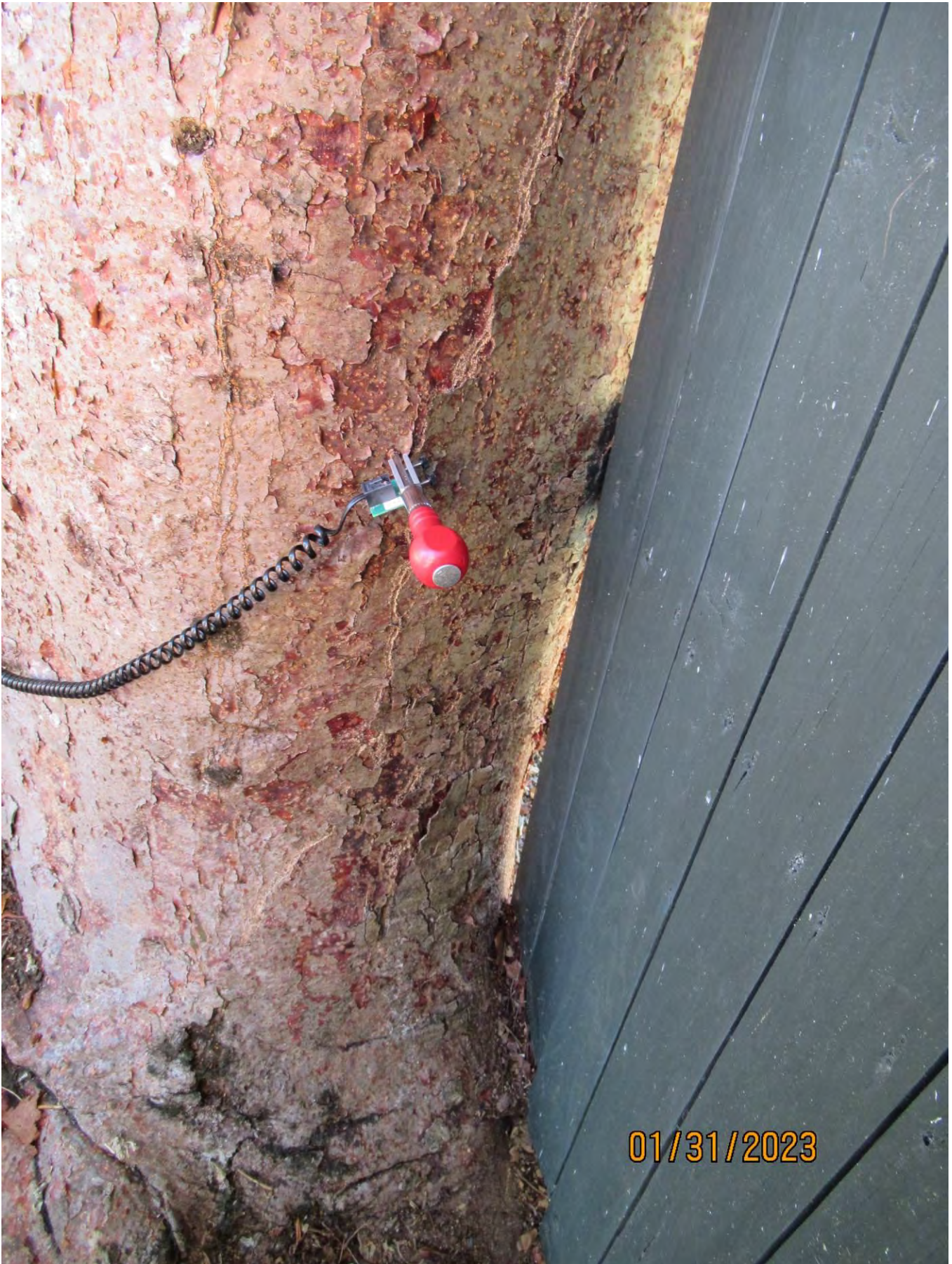
The Tree Check Sonic Wave Tree Decay Detector that the representative for the properties used to measure the decay in the trunk of the tree.
