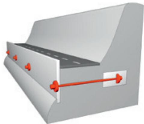
Roadway Embankment Stabilization
