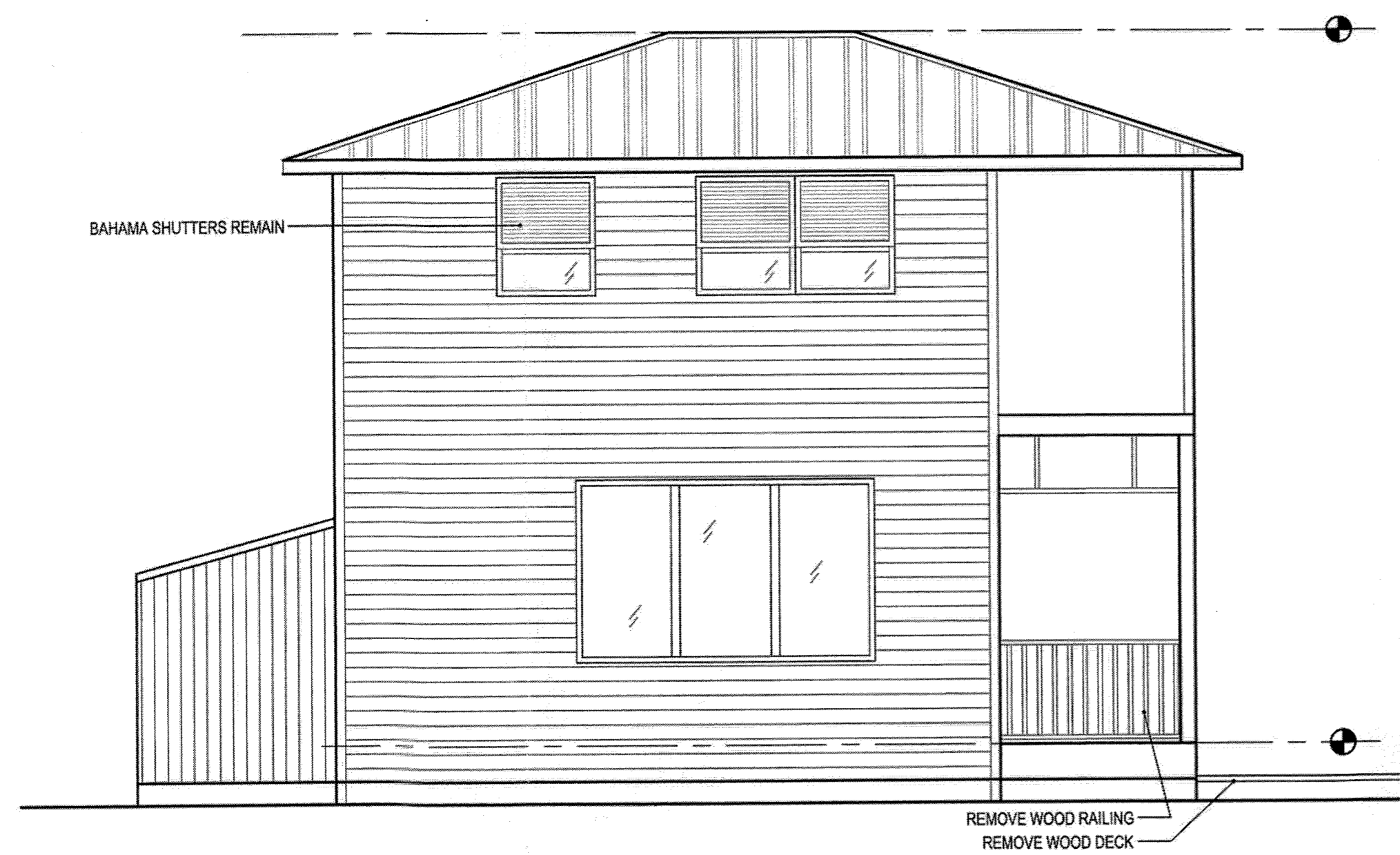
3 EXISTING SOUTH ELEVATION AE3 SCALE: 1/4"=1'-0"
