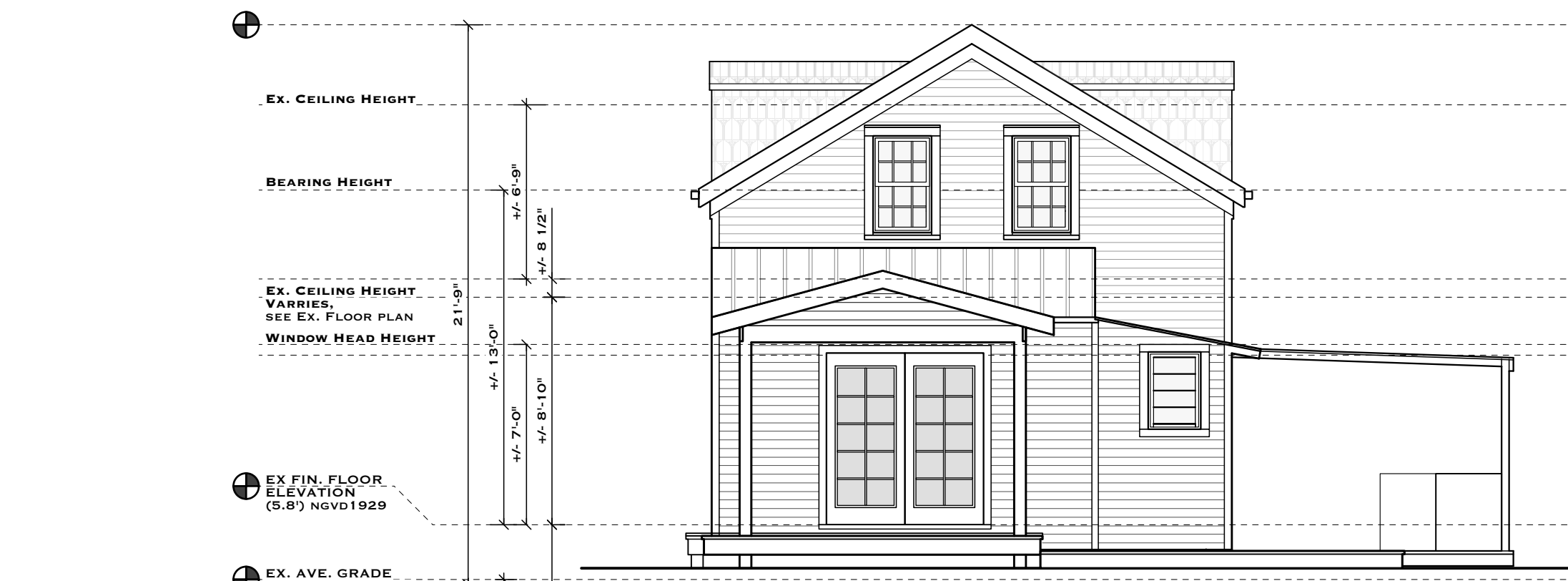
5 EXISTING ELEVATION - REAR (SOUTH) EX1.1 SCALE: 3/16" = 1'-0"
