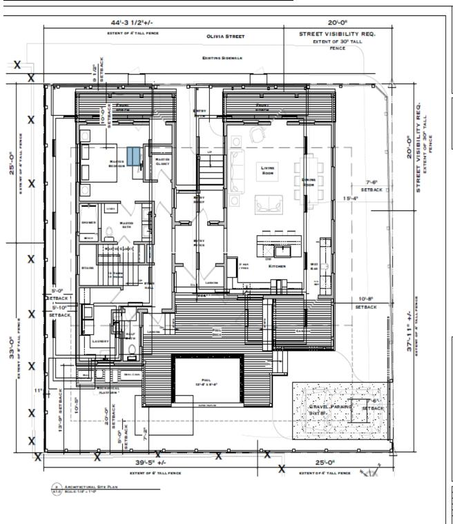
Close up of Rear Set Back dimensions: Features are the same as previous plans except the pool and deck were lowered to 28 1/2", and will not be included in the building coverage. The proposed rear setback variance improves from 7'2" to 13'9".
