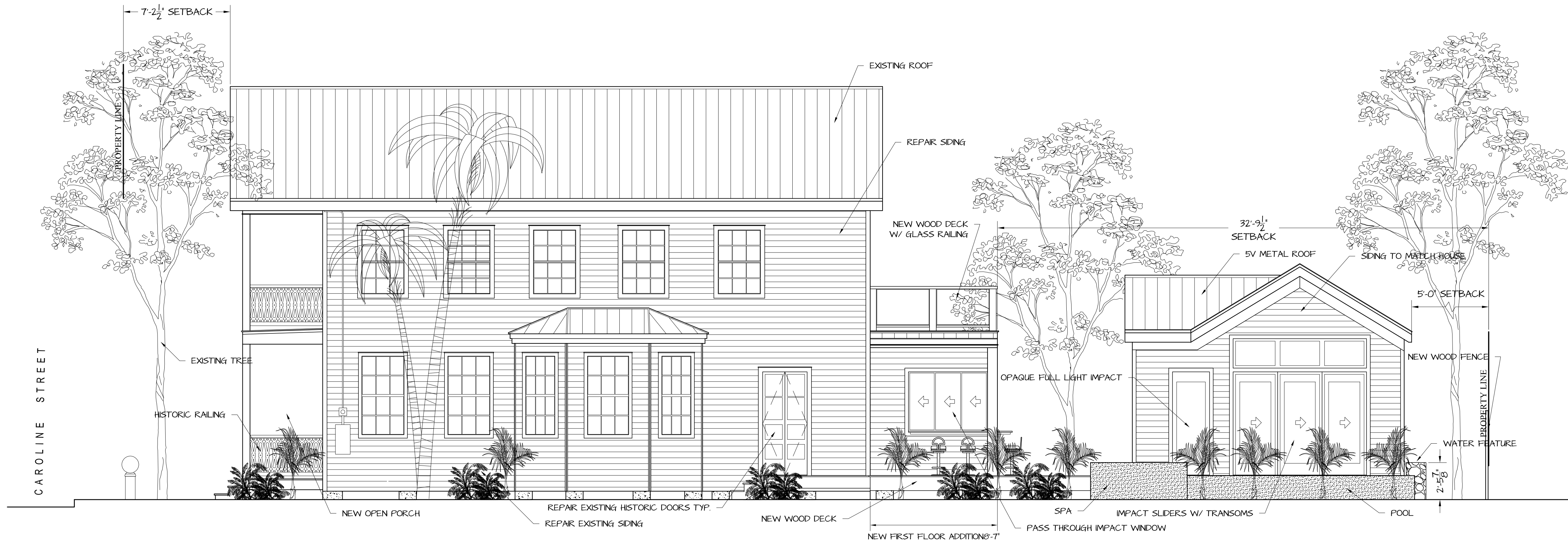
EAST ELEVATION (PROPOSED) 1/4" = 1'-0"
