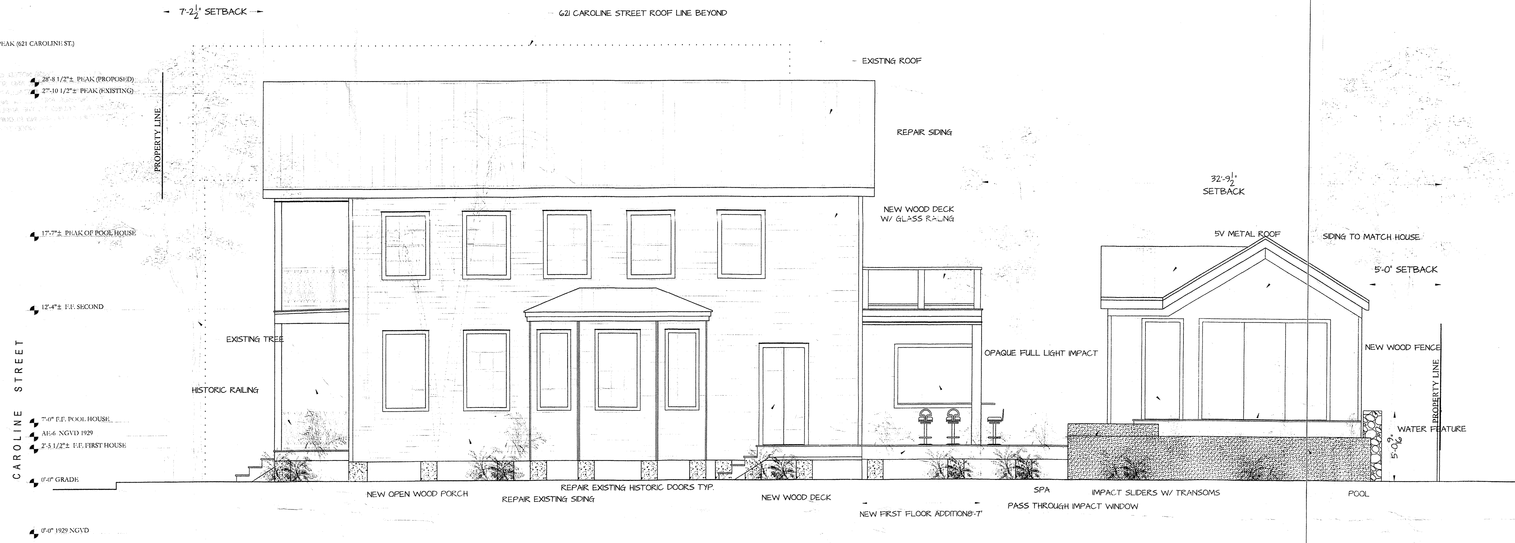
EAST ELEVATION (PROPOSED) 1/4" = 1'-0"
