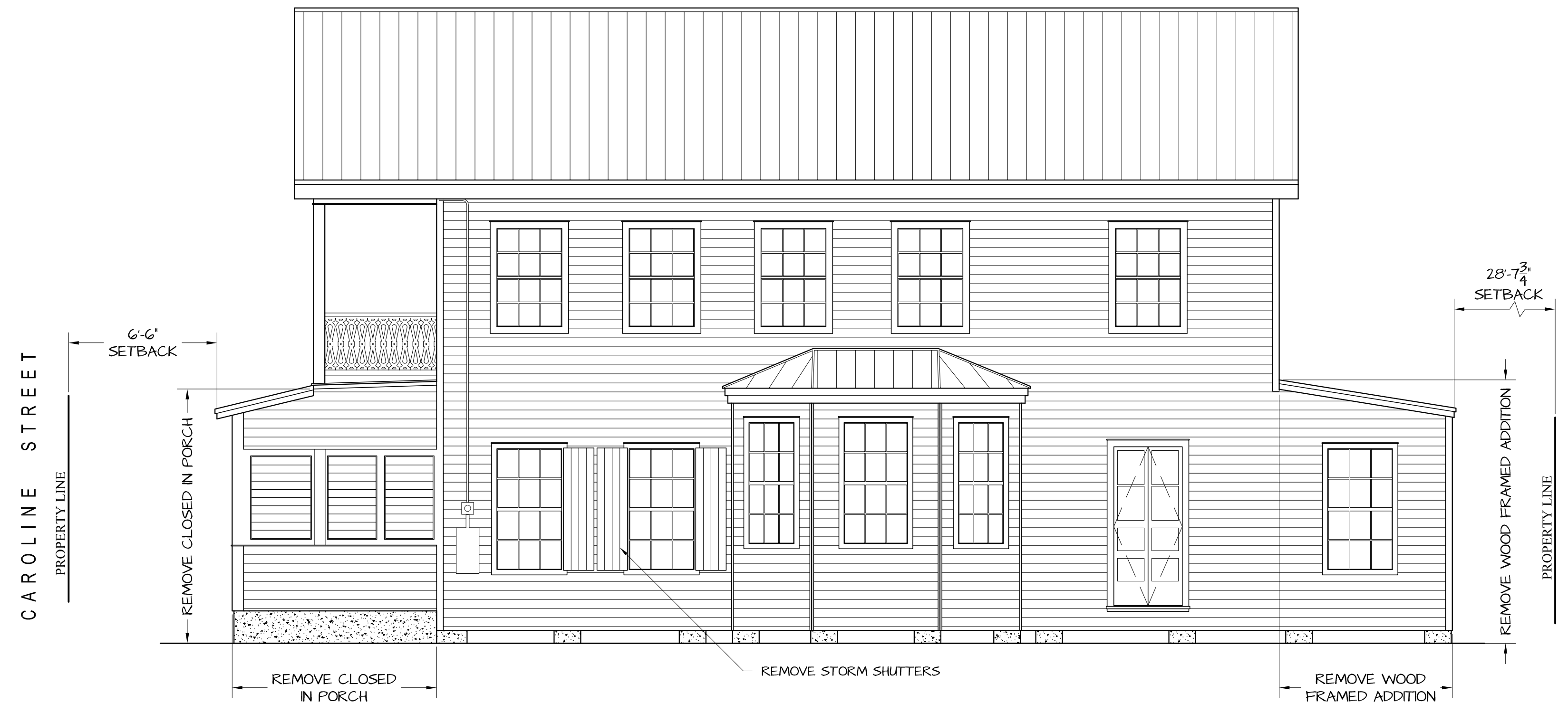
EAST ELEVATION (EXISTING/ DEMO) 1/4" = 1'-0"
