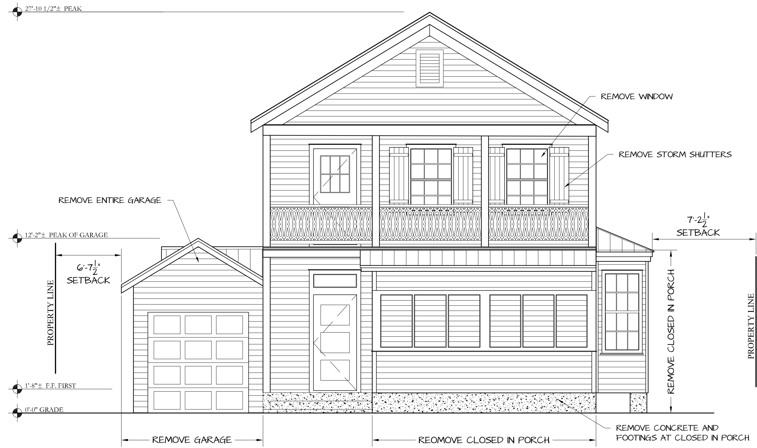
SOUTH ELEVATION (EXISTING/ DEMO) 1/4" = 1'-0"
