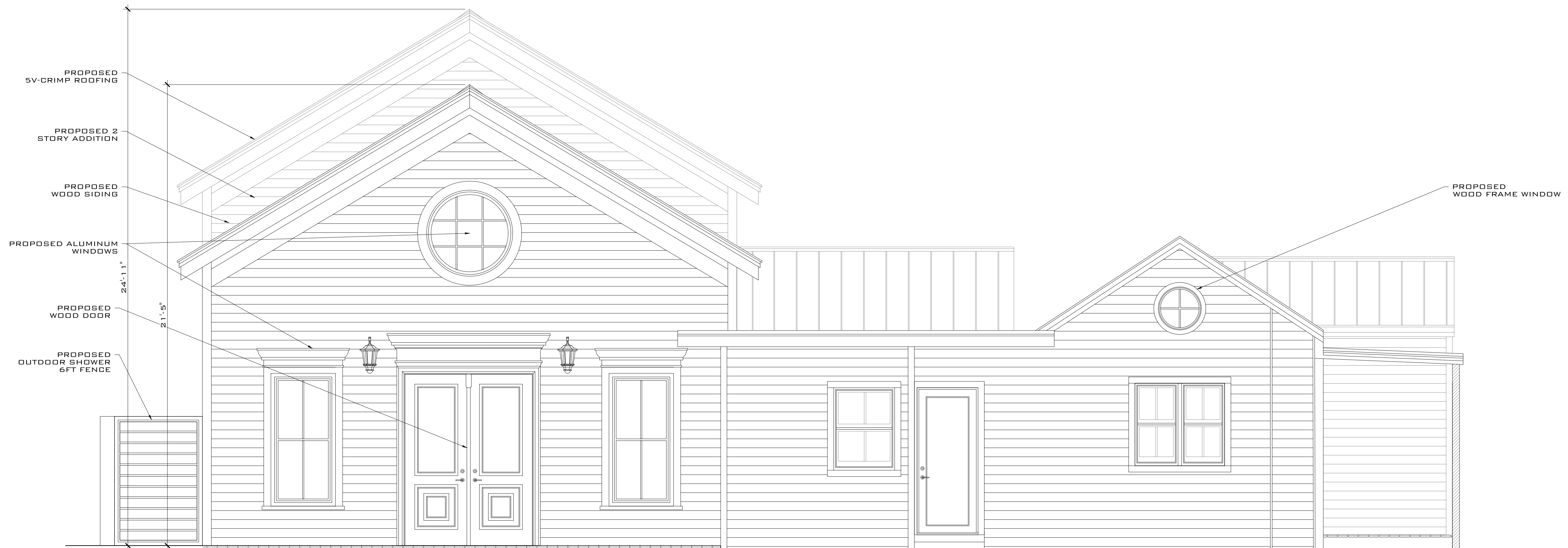
PROPOSED FRONT ELEVATION SCALE: 3/8" = 1'-0"
