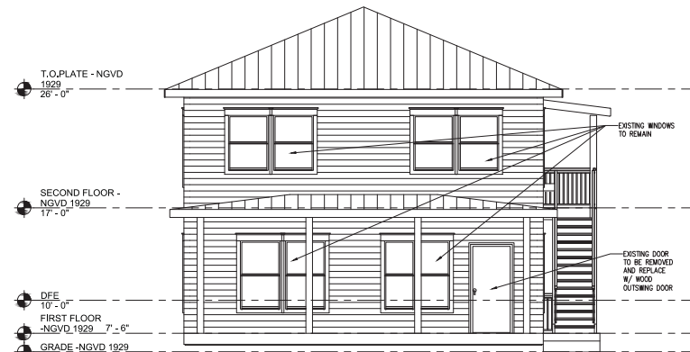
1 PROPOSED FRONT ELEVATION SCALE: 1/4"=1'-0"
