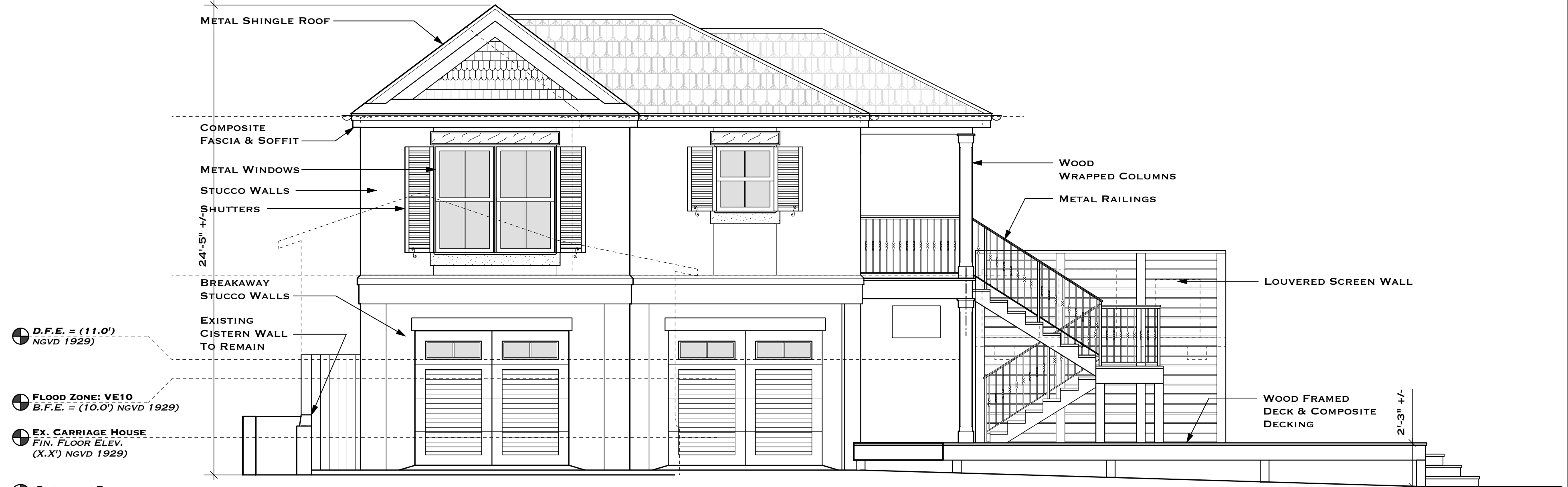
1 WHITEHEAD STREET GARAGE ELEVATION A3.3 SCALE: 1/4" = 1'-0"
