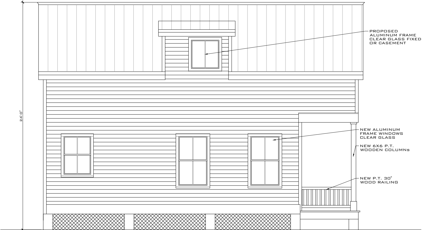
PROPOSED LEFT SIDE ELEVATION
