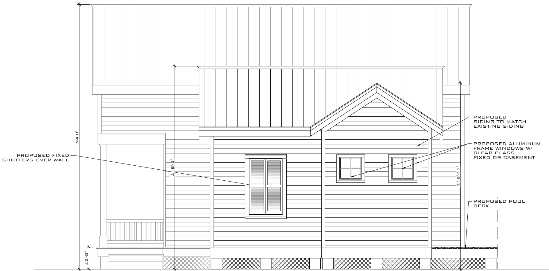
PROPOSED RIGHT SIDE ELEVATION
