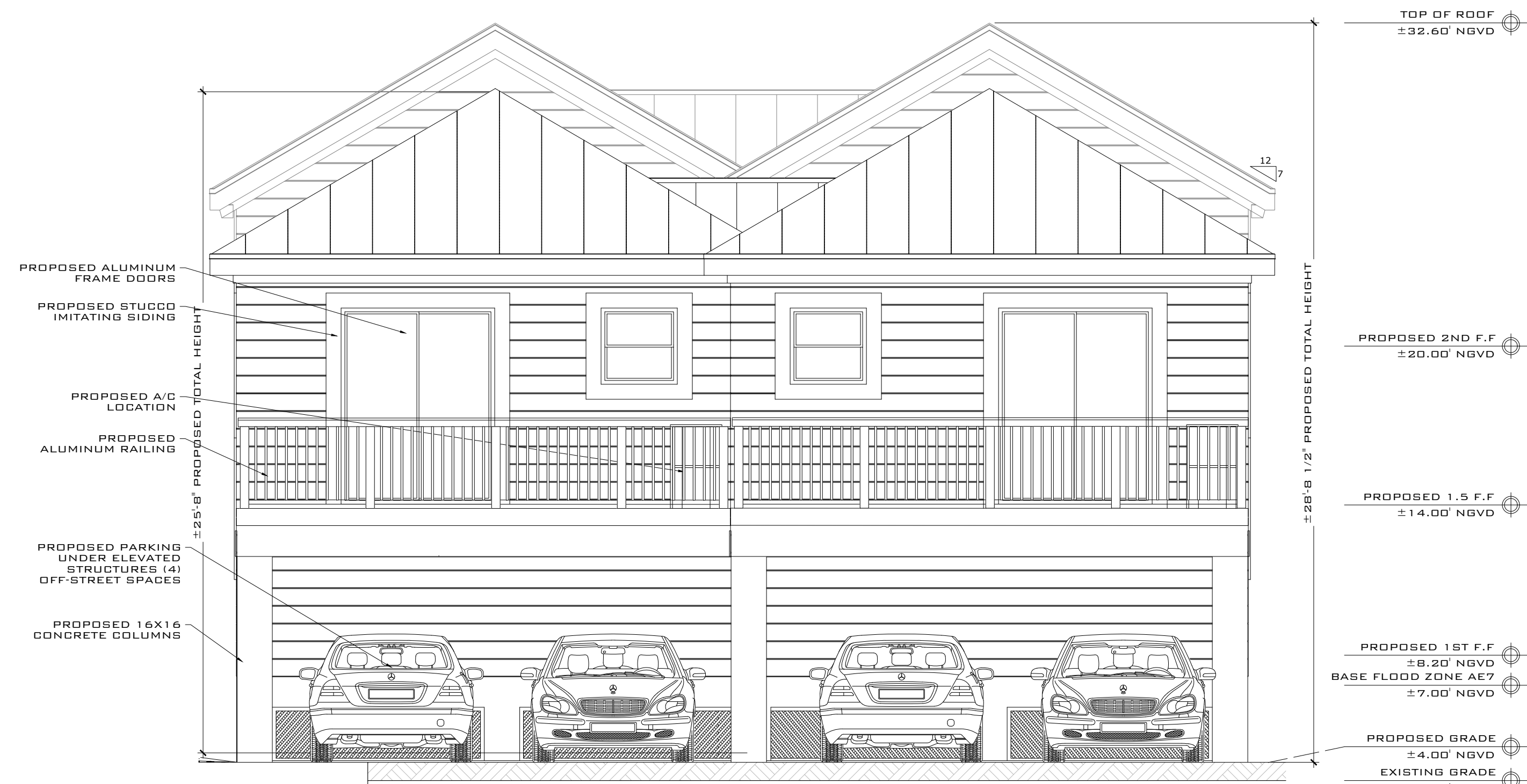
PROPOSED STREET SIDE ELEVATION SCALE: 1/4" = 1'-0"
