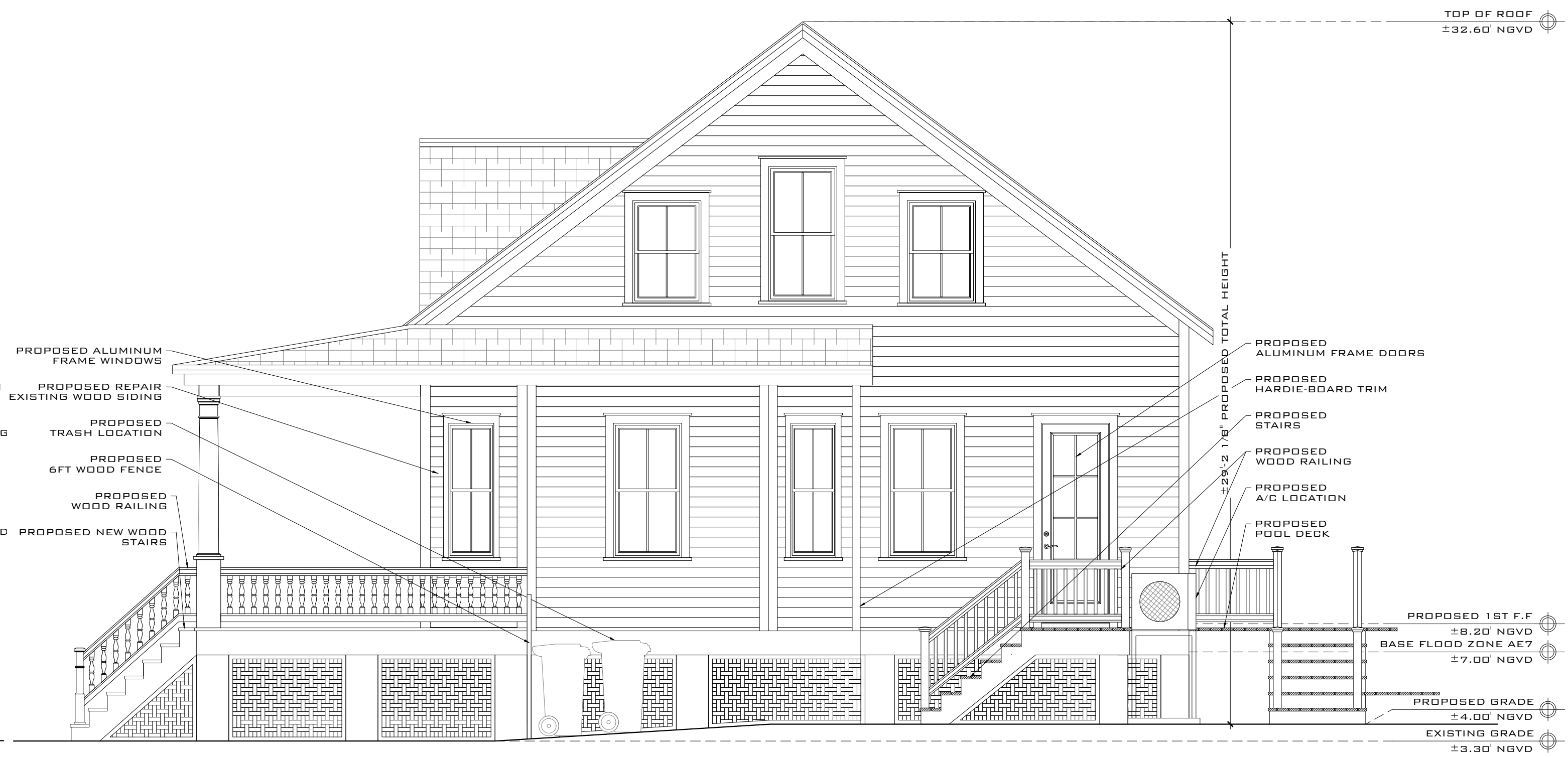
PROPOSED RIGHT ELEVATION SCALE: 1/4" = 1'-0"
