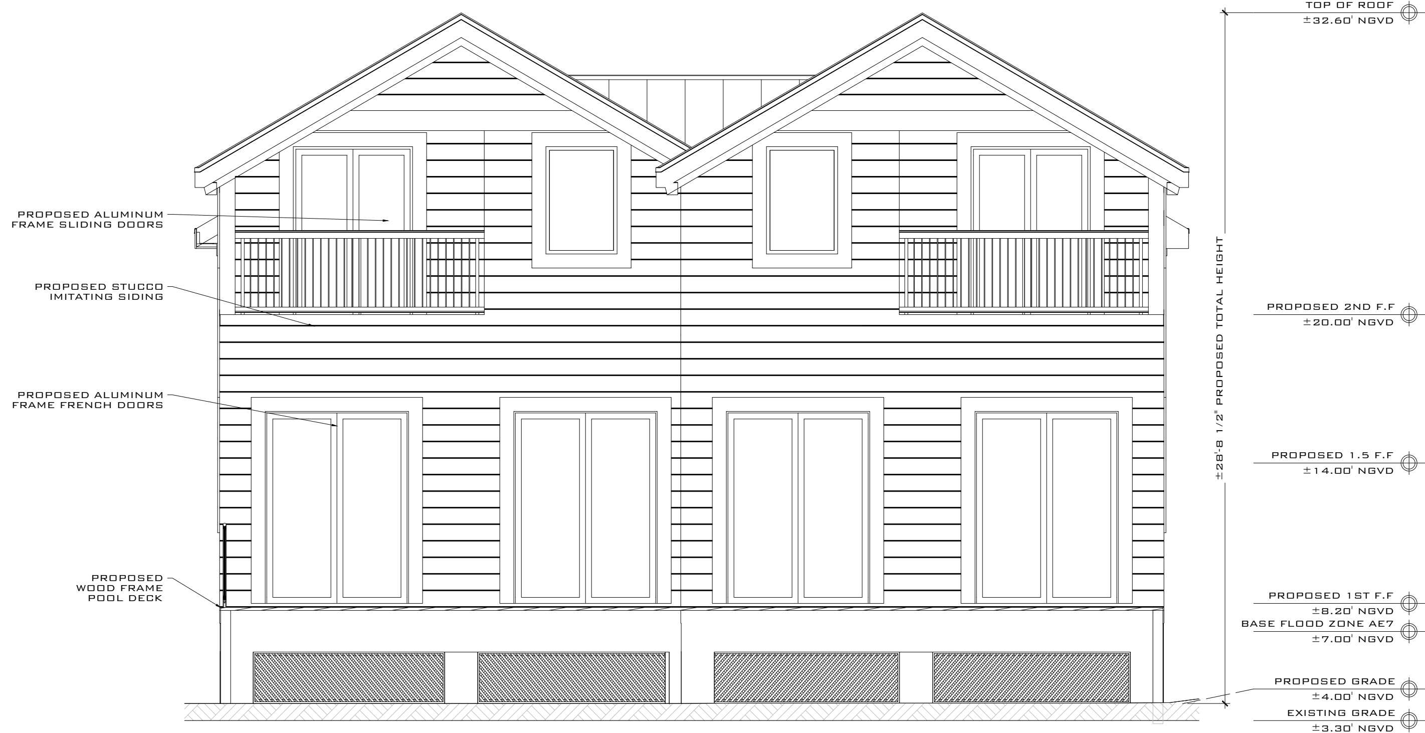
PROPOSED FRONT ELEVATION SCALE: 1/4" = 1'-0"
