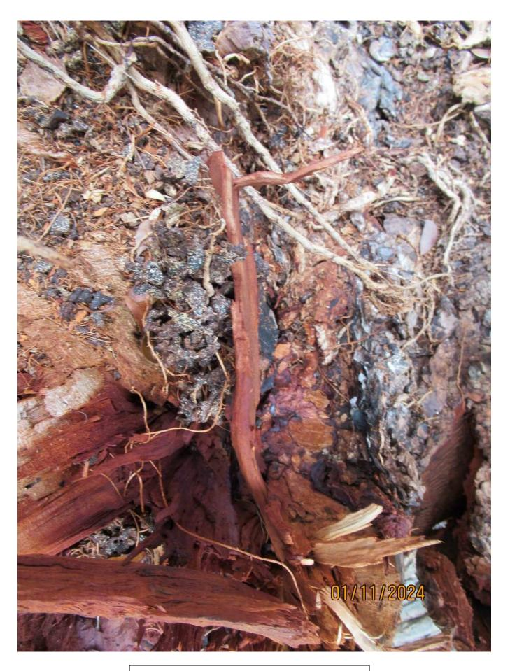
Closeup photo of tear area showing termite dirt.
