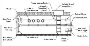
Water Reservoir tank is a pre-cast Concrete vessel with lockable access hatch, service ladder and required plumbing connection Tanks manufactured of 5000 PSI concrete to meet ASTM C-913 & C-1227 standards. Tank size to be per project requirements based on splash pad feature flow rate, size of pad, and environmental surroundings.
