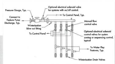
Distribution Manifolds are preplumbed water delivery systems from feature pumping system to water play features. Standard distribution manifolds consist of manual flow control valves that regulate water flow levels to each water element for on/off control systems. When creating water play zones or sequencing water play activities, standard distribution manifolds can be upgraded with electric valves or solenoid valves.
