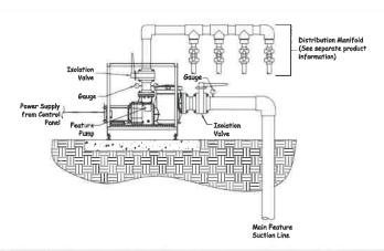
Feature Skid to be UL listed system capable of flow rates from 250 gpm to 3000 gpm. System equipment to be pre plumbed using all schedule 80 PVC pipe & fittings and mounted on a epoxy painted steel skid with adjustable leveling legs. System to be tested prior to shipment
