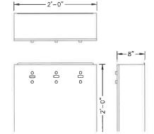
Control Panels are used to control simple on/off operations of water play activities or incorporate operation interface Programmable Logic Controller, (PLC), to create splash pad zoning or sequencing activities.
