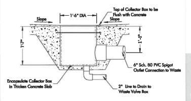
Collector Box to consist of 18 inch diameter PVC sump for collection of splash pad recirculation water. Each collector box is capable of 250 gpm gravity drainage using a 6 inch drain pipe sloped at 1/8 inch per foot slope to water reservoir tank
