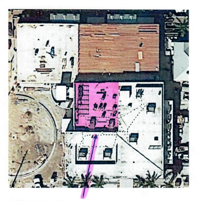
Roof area to be repaired and recoated with silicone sealant
