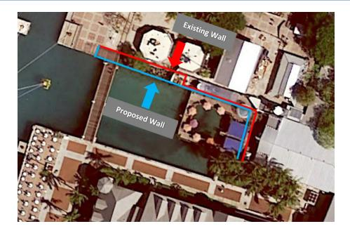
Construction of the east wall may require demolition of a portion of the pile supported concrete turtle tanks, and that work will be coordinated with the City. Any work on the east wall will be parceled out as an alternative bid item to keep the Irma damaged north wall segregated from any extra work not considered to be damaged by Hurricane Irma.
