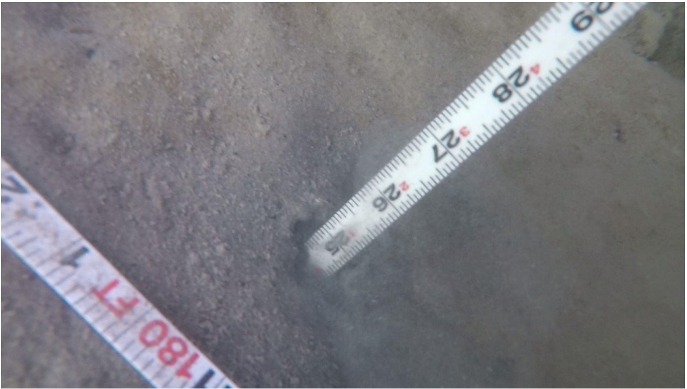
Underwater 21 - at 180ft the soft sediment is 25in deep
