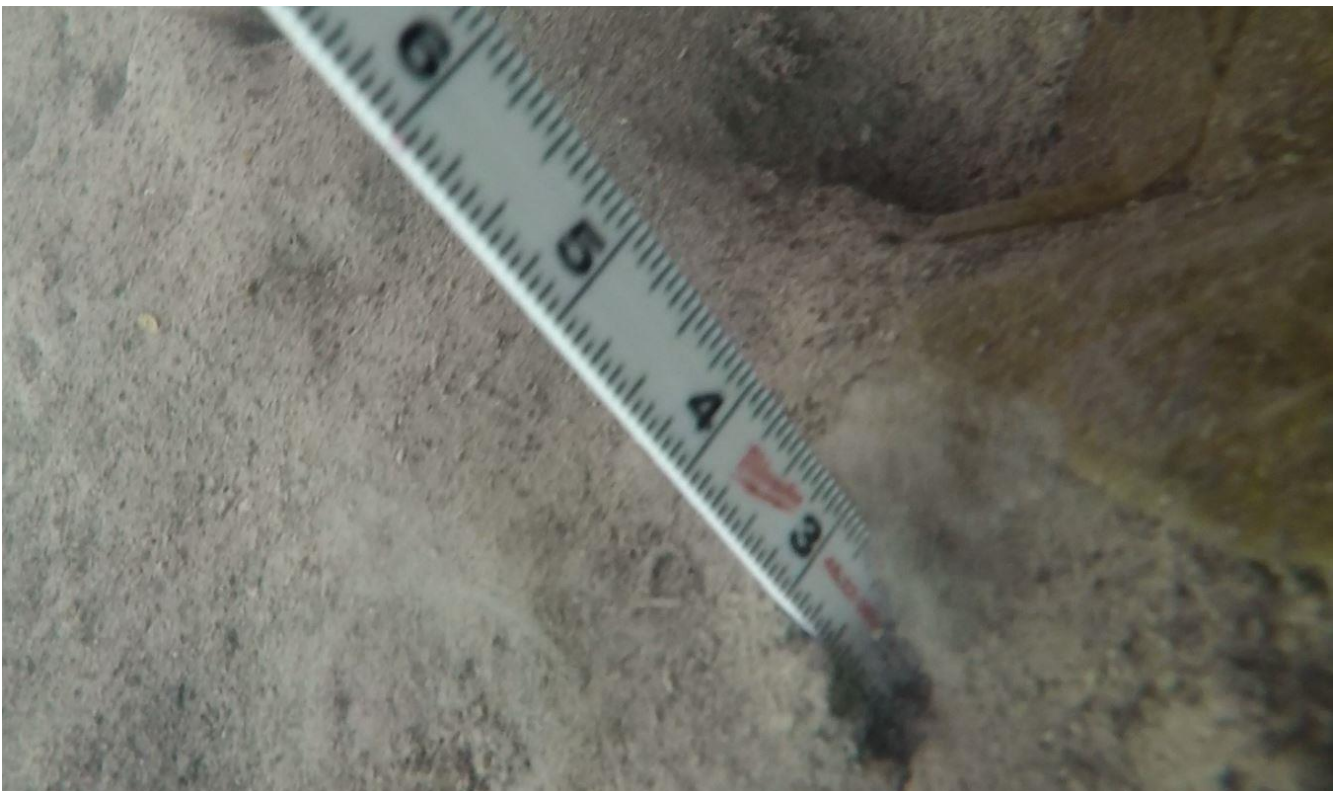
Underwater 12 - at 69ft shows sediment thickness at approximately 3in
