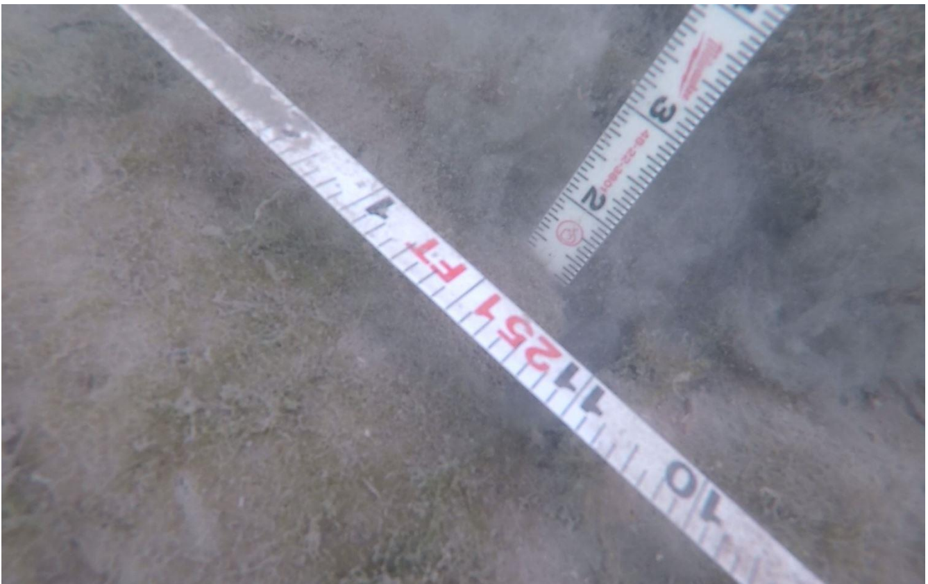
Underwater 26 - at 251ft shows 1in of sediment at toe
