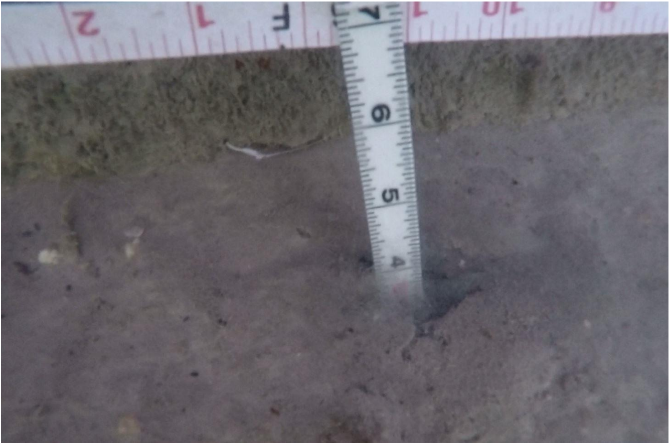
Underwater 37 - at 350ft showing 4in sediment
