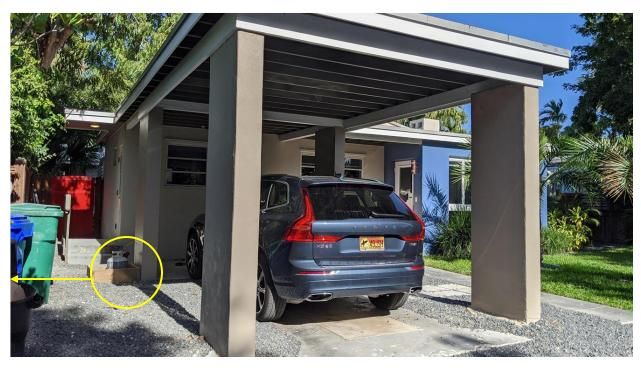
The temporary propane tank location will be relocated to meet fire requirements to the left of the of the property line. The final installation will include a concrete slab, and a 4-foot-high propane tank tied to the slab.
