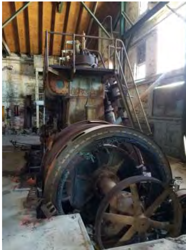
Nordberg Dynamo generator in Building 2
