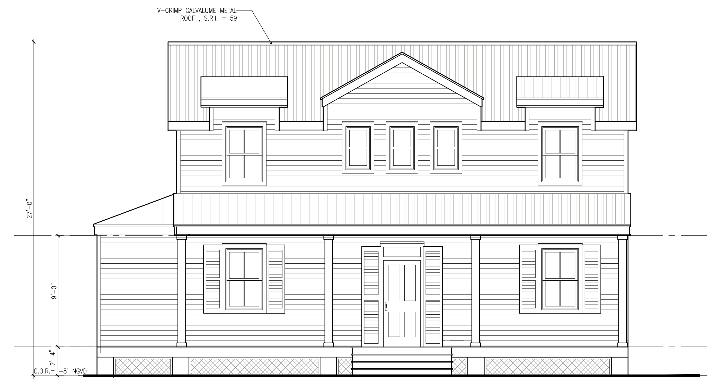
4 UNIT 2 EAST ELEVATION A2.31 SCALE: 1/4"=1'-0"
