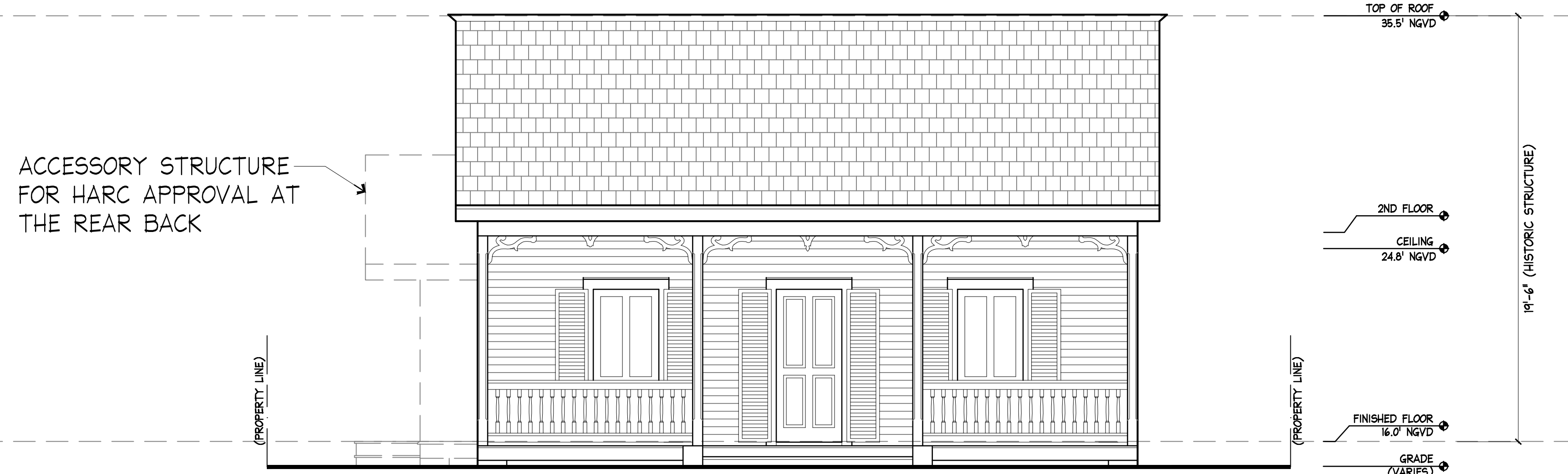
1 PROPOSED SOUTH ELEVATION A4 SCALE: 1/4"=1'-0"
