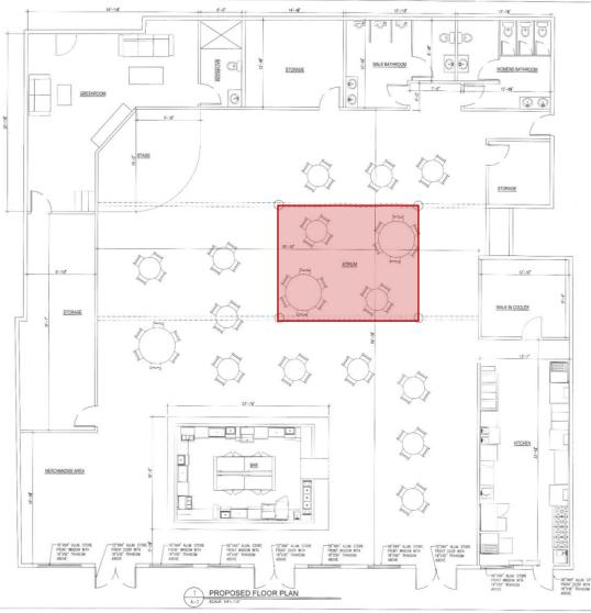
The applicant has proposed to convert the retail use of the structure а to restaurant use. The proposed project would redevelop and reconstruct the structure and add floor additional area outlined in red.
